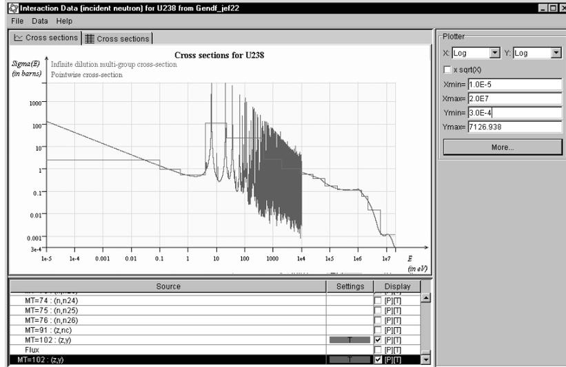
Fig. 4 Comparison of pointwise and multi-group cross-sections
