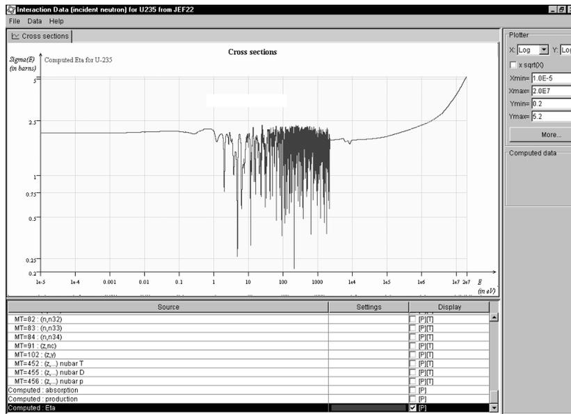
Fig. 5 Example of cross-section manipulation  $\eta = (v \sigma_f / \sigma_a)$
