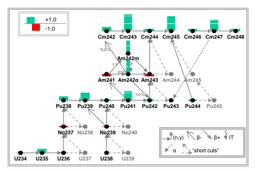
Figure 1: MA/Pu = 1; ω-values comparison: burn-up chain implemented in the ERANOS code
