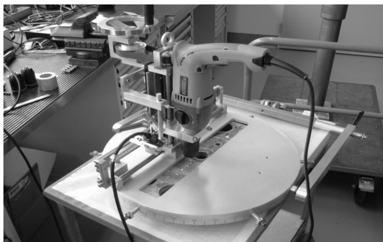
Figure 7: Drilling device to retrieve LBE samples from the target sample pieces
