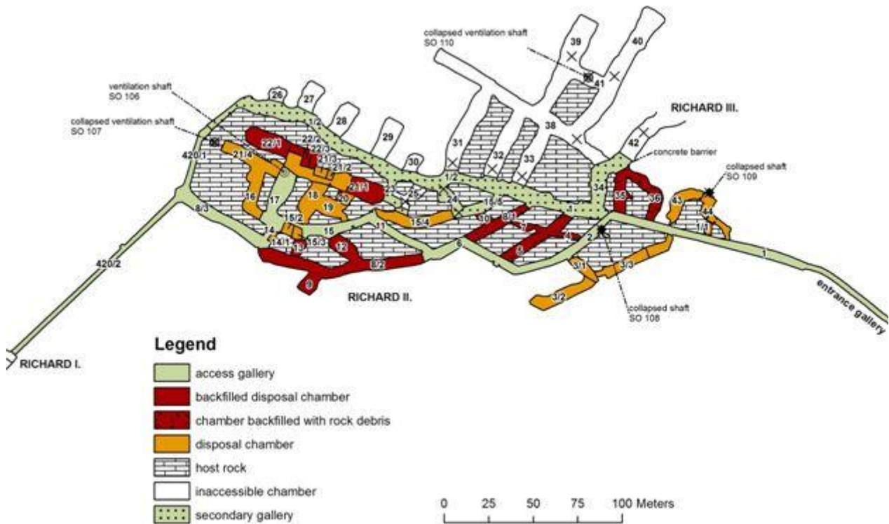
The repository **Bratrství** is located in a former uranium mine near the town of Jáchymov and is designed for disposal of waste containing naturally occurring long-lived nuclides only, such as  $^{226}\text{Ra}$  and uranium. Its disposal capacity is approx. 1 200 m<sup>3</sup>, from which is free approx. 340 m<sup>3</sup>. In 2012 the chamber 2 was sealed with special concrete backfill. Sealing of the remaining chambers will follow.
