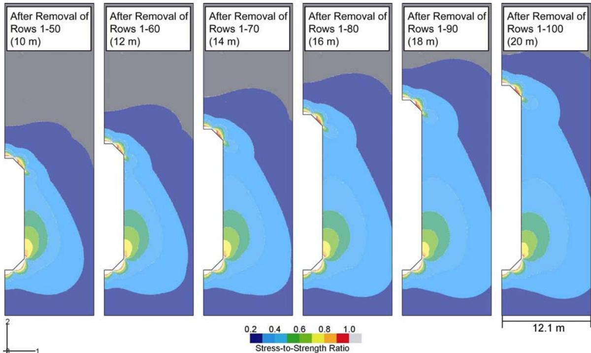
Effects of Progressive Spallation on Overstress Distribution Around A Thermally Loaded Drift. Spallation was Simulated Through Removal of Rows of Rock Elements in the Roof, One Row at a Time
