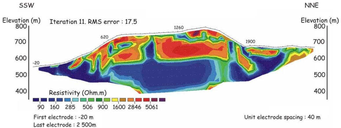
In the WNW-ESE oriented Southern profile (Figure 3), a large more conductive zone is seen between points 920 and 1 340 m, borders zone may be associated with faulted material. The N-S-trending and N130-trending fault zones seen from the tunnel (Cabrera *et al.*, 2001) (Figure 1) could correspond to fault zones identified around the point 1 340 m in Figure 3.
