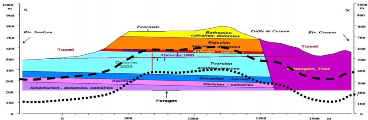
A secondary fault zone was intercepted in clays by several drifts and boreholes from the tunnel. This hectometre-sized sub-vertical fault set, displaying a 2 m vertical offset and larger horizontal offset, presents significant variations of aspect, from a dry metre-sized fault gouge showing the same aspect as intact rock, to a draining breccia associated with a 10 m wide fractured zone.
