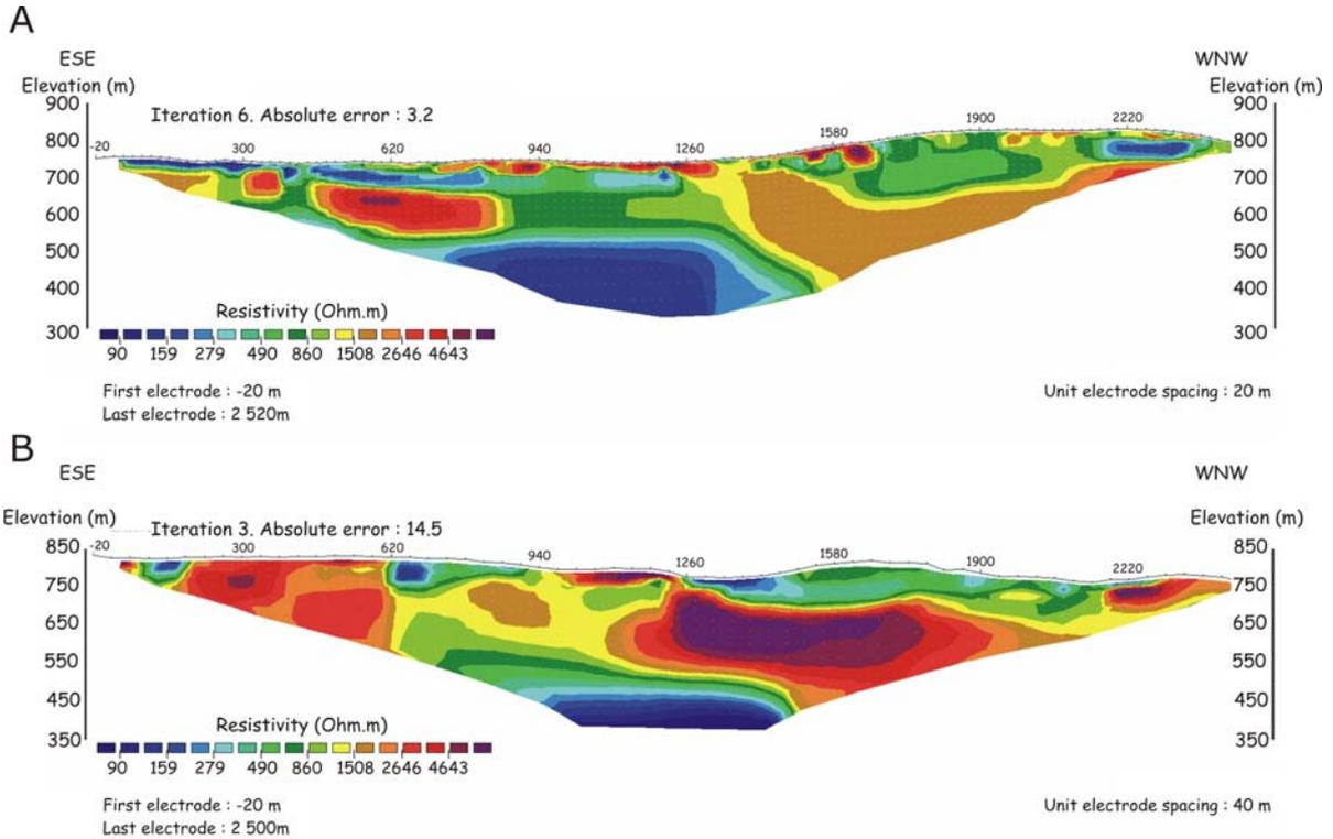
Figure 4. Electrical resistivity image after inversion (L2 norm) of Wenner-Alpha configuration data. The argillite layer location is imposed in the inversion
