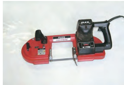
Handheld mechanical cutting equipment for small contaminated pipes, conduit and ducting. BR-3 decommissioning project, Mol, Belgium. [Photos: SCK•CEN]
