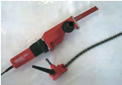
Handheld mechanical cutting equipment for small contaminated pipes, conduit and ducting. BR-3 decommissioning project, Mol, Belgium. [Photos: SCK•CEN]
