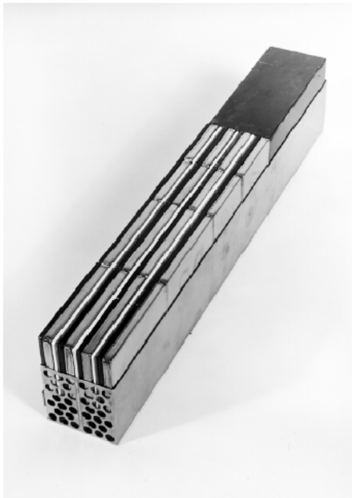
Figure 1.1.8. Typical Loaded Drawer* (The plates are elevated above the bottom of the drawer in this photograph.)
