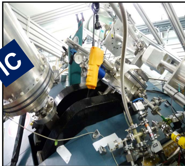
Ionisation Chamber (IC) used for the mass Yield measurement: Y(A)
