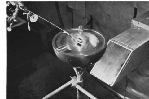
FIG. 9.3.—Source plate and a spiral counter in position at the centre of a hemisphere.
