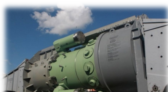
Transporting the RITM-200 steam generating unit
