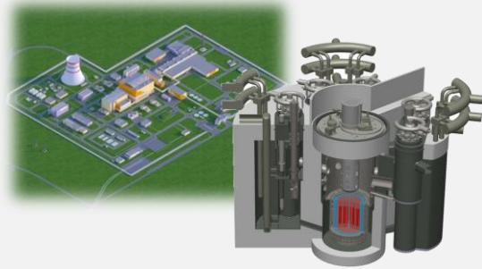
Pilot Demonstration Energy Complex with BREST-OD-300 Reactor
