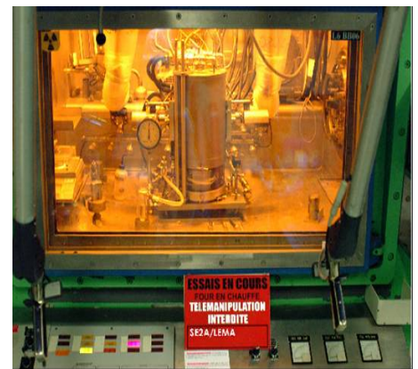
Figure 4. High temperature oven in a shielded hot cell
