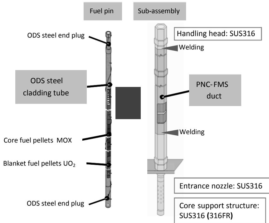
**Figure 8: Material selection for major components of the JSFR**
