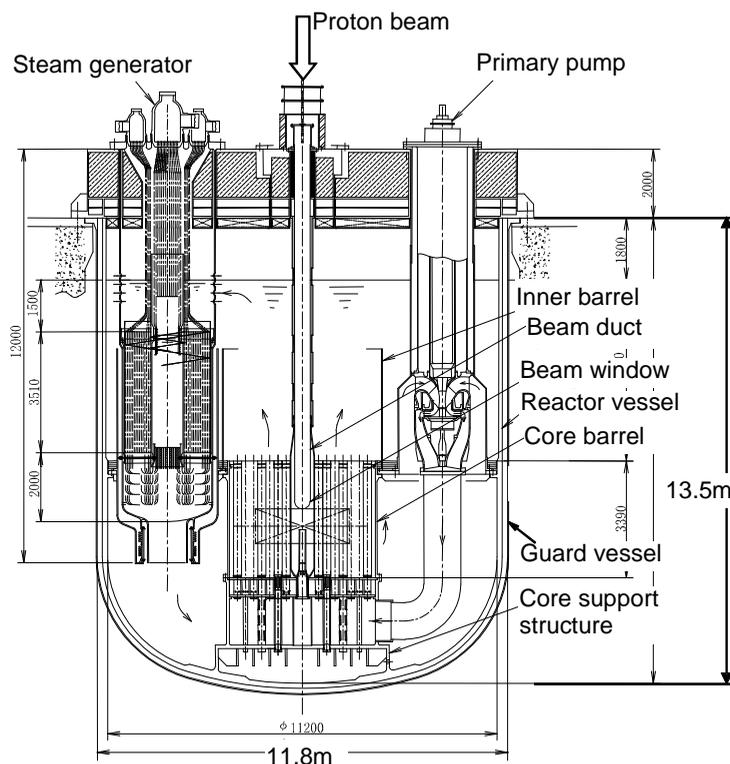
Neutrons generated by the 1.5 GeV proton beam induced to the spallation target (lead-bismuth) burn the nitride fuels (MA+Pu)N+ZrN) in this reactor. Steam is generated by the SG in the RPV. Initial MA inventory is 2.5 tonnes and 250 kg of MA are transmuted yearly. MA-containing fuel is exchanged after 600 EFPD. Thermal output of the reactor is 800 MWth and predicted reactor lifetime is 40 years.
