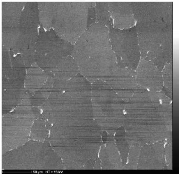
Note: The light contrast at the grain boundaries correspond to tungsten precipitates.
