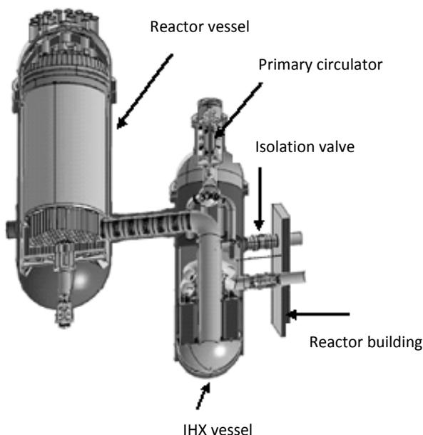
**Figure 2: Gas-cooled fast reactor: The ALLEGRO primary system overview [7]**
