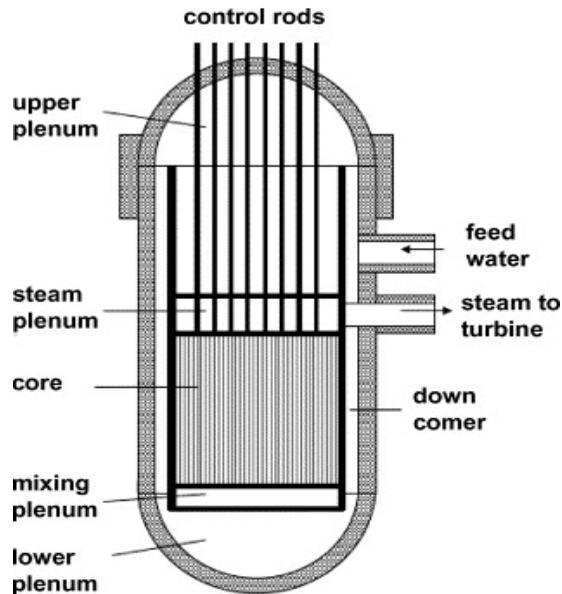
Figure 16: Design of the assembled RPV with internals [3]
