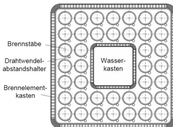
Brennstäbe = fuel rods; Drahtwendelabstandshalter = wired fuel rod spacer;
