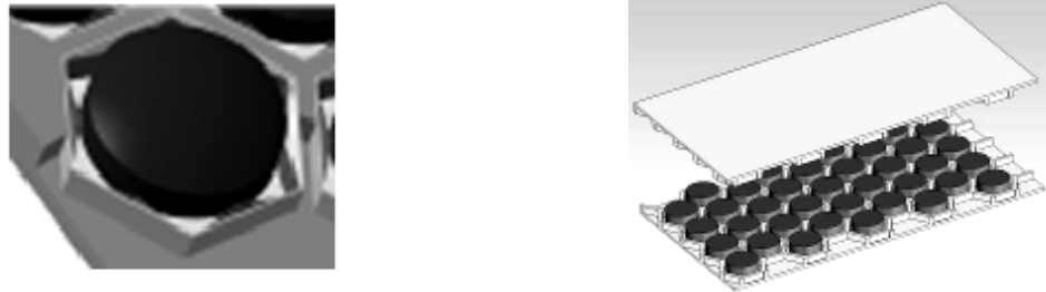
Figure 2.2 View of the fuel plate type element for GFR, made of two ceramic plates enclosing a honeycomb structure containing cylindrical pellets made of the mixed carbide
