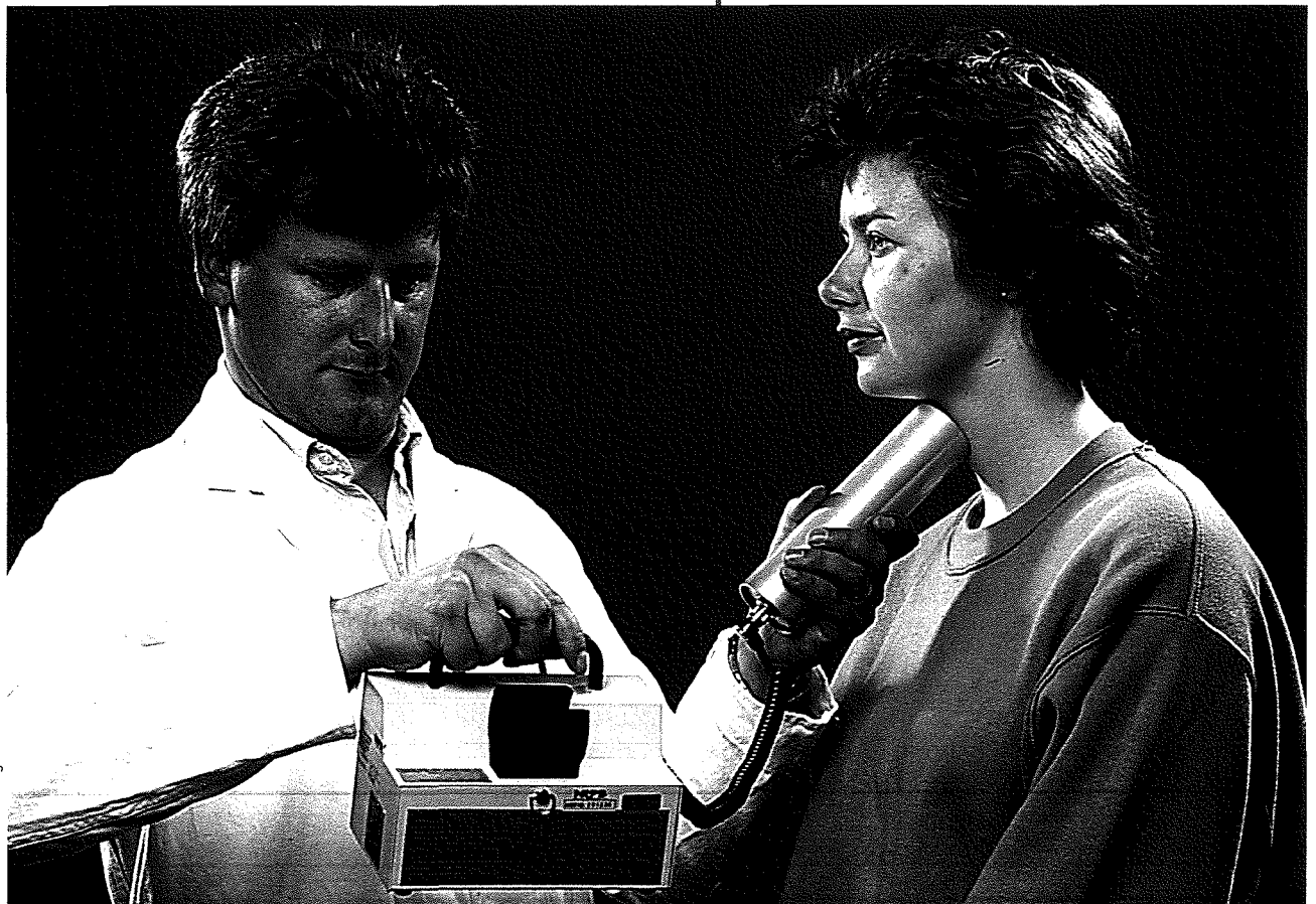
Monitoring for the presence of radioactive iodine in the thyroid gland. The instrument measures the gamma radiation given off by the iodine.
