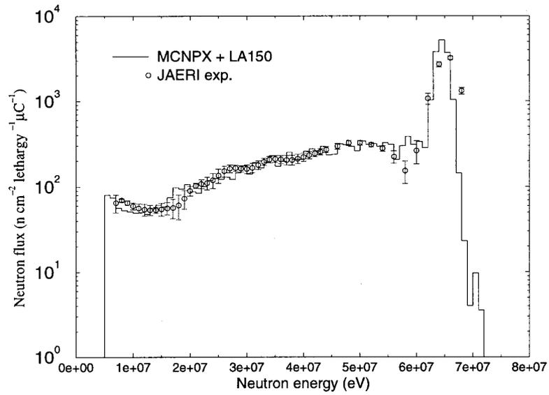
**Figure 3. 68 MeV neutrons on 40 cm of iron, detector at 20 cm**
