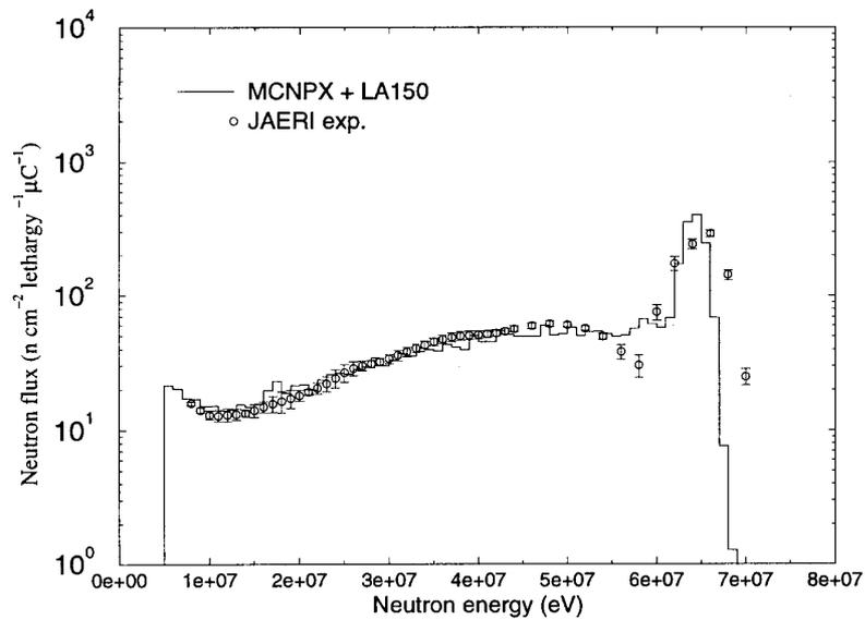
**Figure 4. 68 MeV neutrons on 40 cm of iron, detector at 40 cm**
