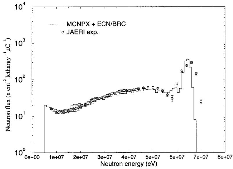
**Figure 7. 68 MeV neutrons on 40 cm of iron, detector at 40 cm**
