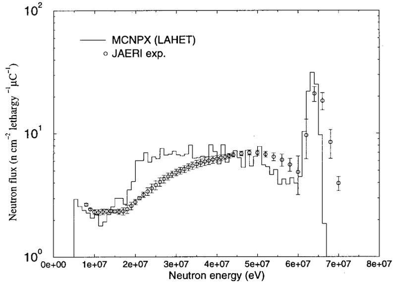
**Figure 11. 68 MeV neutrons on 40 cm of carbon, nitrogen and oxygen, detector at centreline**
