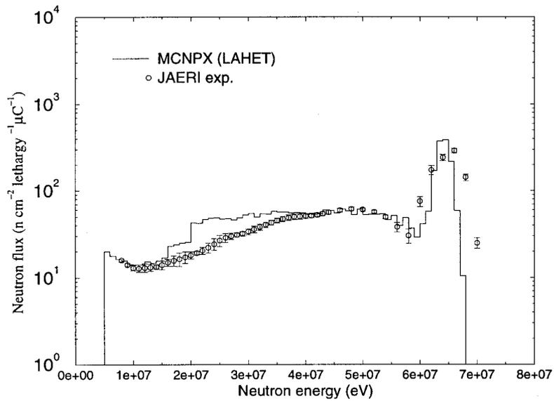
**Figure 10. 68 MeV neutrons on 40 cm of iron, detector at 40 cm**
