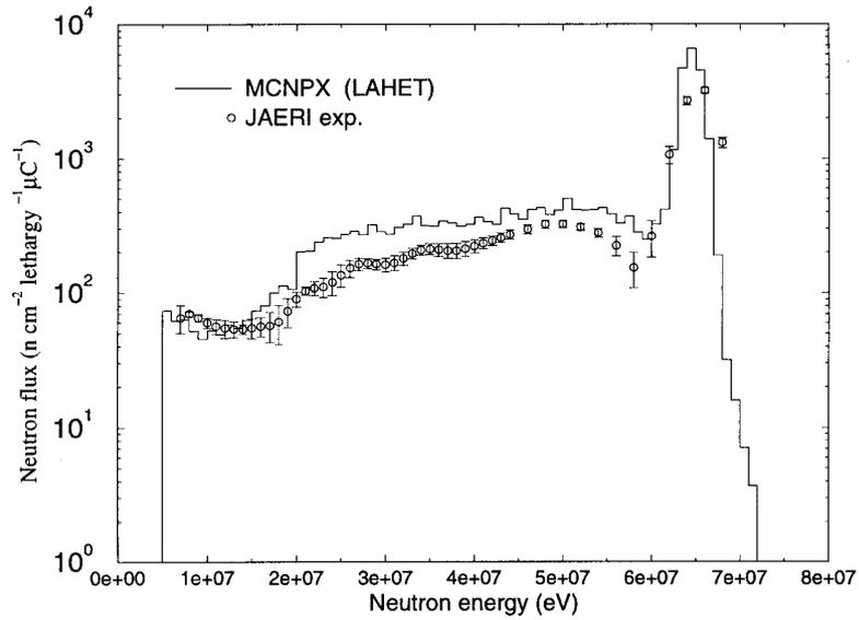
**Figure 9. 68 MeV neutrons on 40 cm of iron, detector at 20 cm**
