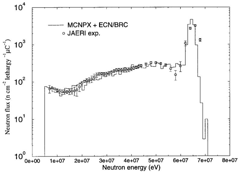
**Figure 6. 68 MeV neutrons on 40 cm of iron, detector at 20 cm**
