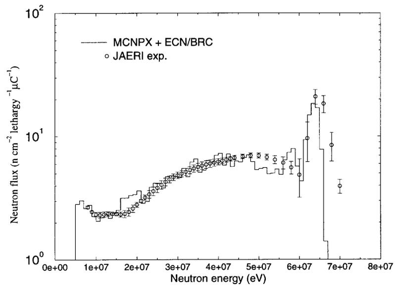
**Figure 8. 68 MeV neutrons on 40 cm of iron, detector at centreline**
