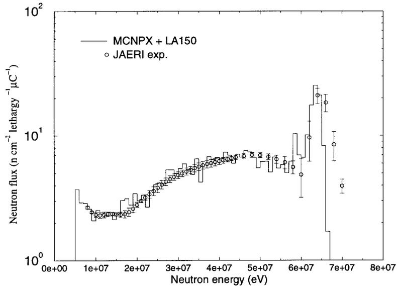
**Figure 5. 68 MeV neutrons on 40 cm of iron, detector at centreline**
