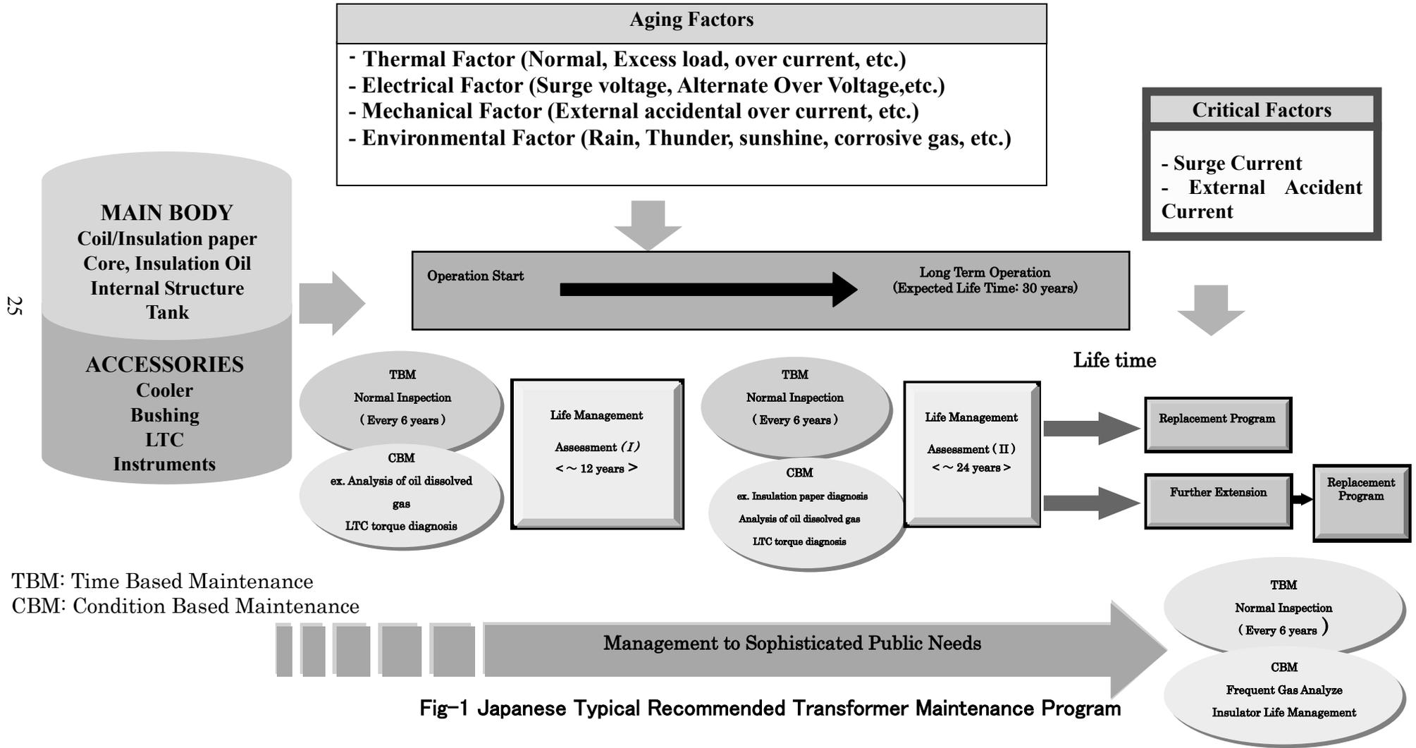
Fig-1 Japanese Typical Recommended Transformer Maintenance Program
