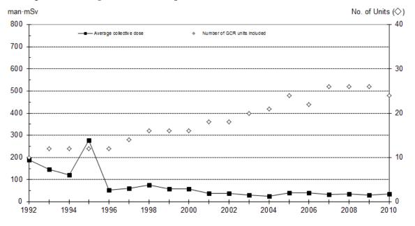
Figure 10. Average collective dose per shutdown reactor: GCRs (man·mSv/reactor)
