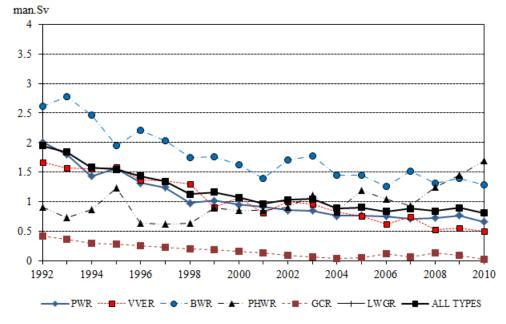
Figure 1. Average collective dose per reactor for all operating reactors included in ISOE by reactor type, 1992-2010 (man·Sv/reactor)
