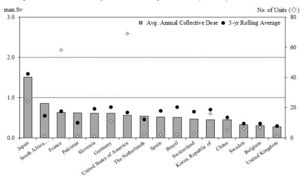
Figure 3. 2010 PWR average collective dose per reactor by country (man·Sv/reactor)
