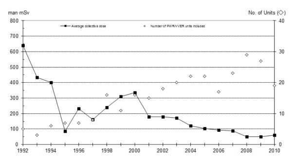
Figure 8. Average collective dose per shutdown reactor: PWR/VVERs (man·mSv/reactor)
