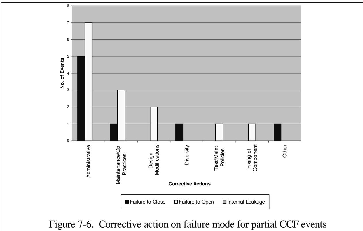
Figure 7-6. Corrective action on failure mode for partial CCF events
