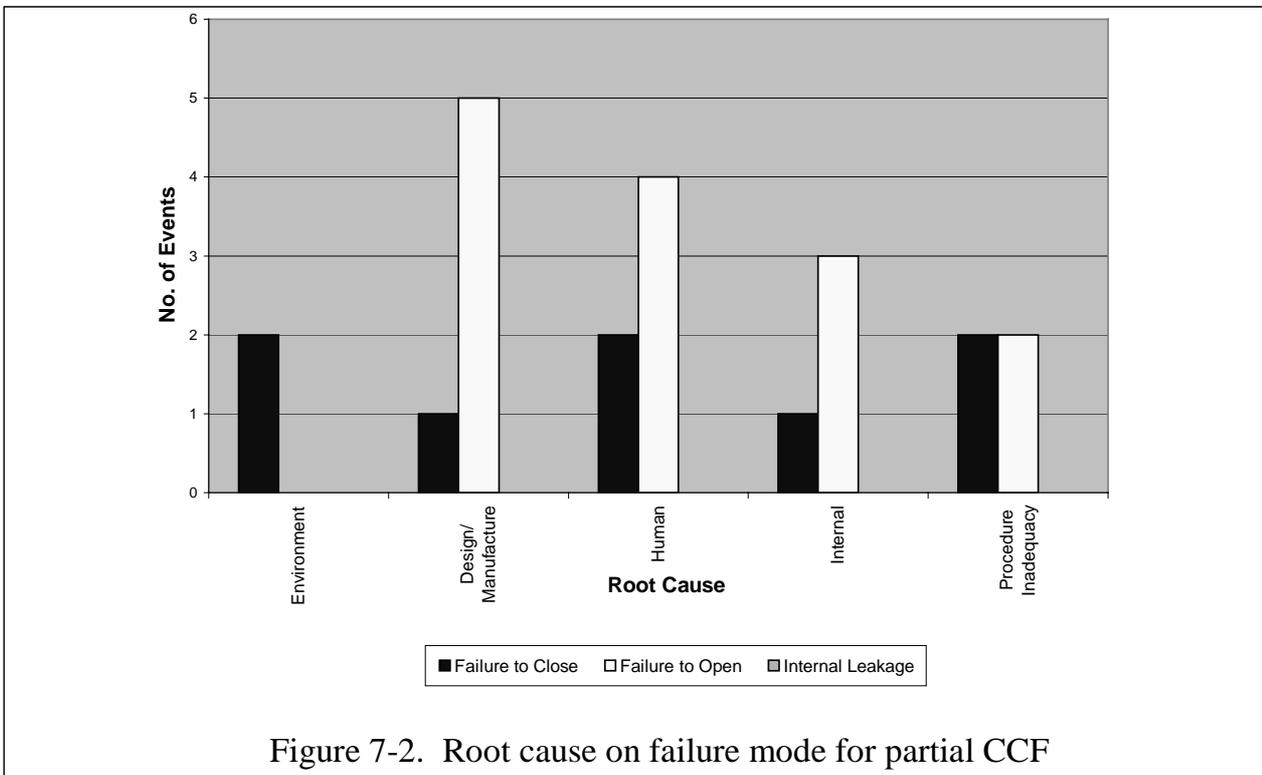
Figure 7-2. Root cause on failure mode for partial CCF
