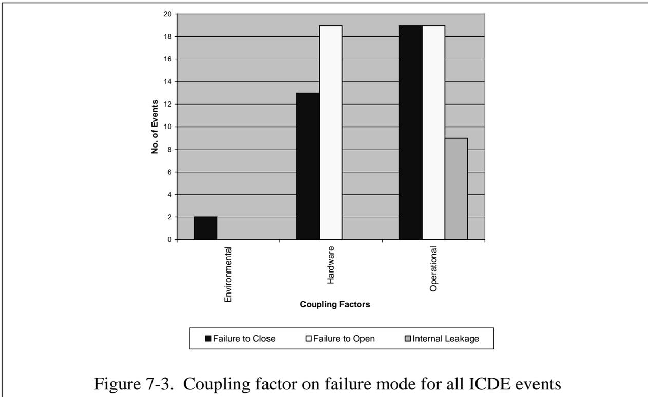
Figure 7-3. Coupling factor on failure mode for all ICDE events
