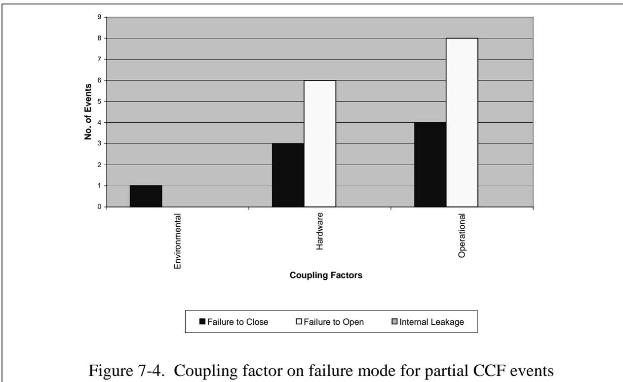
Figure 7-4. Coupling factor on failure mode for partial CCF events
