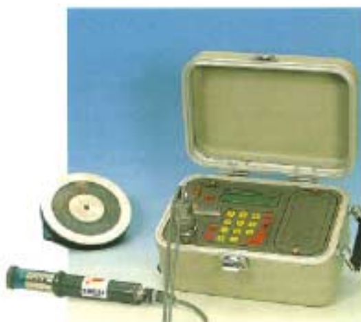
Figure 5.1. Aspect of a portable corrosion rate meter making use of a modulating guard ring.
