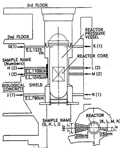
Fig. 1 Sampling location of the concrete core
