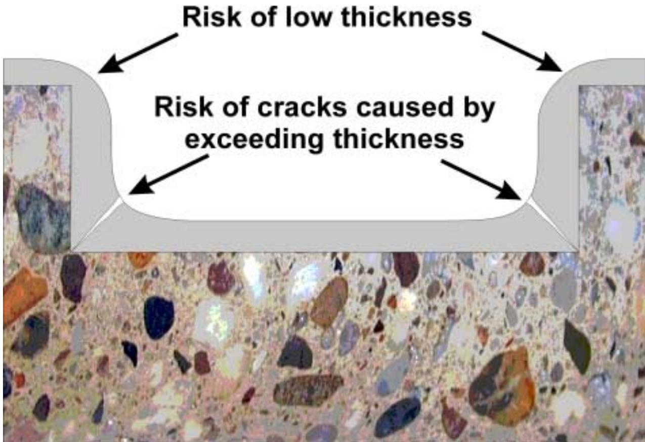
Picture 3: Cross – section of a fluting, showing minimal and excess material thickness
