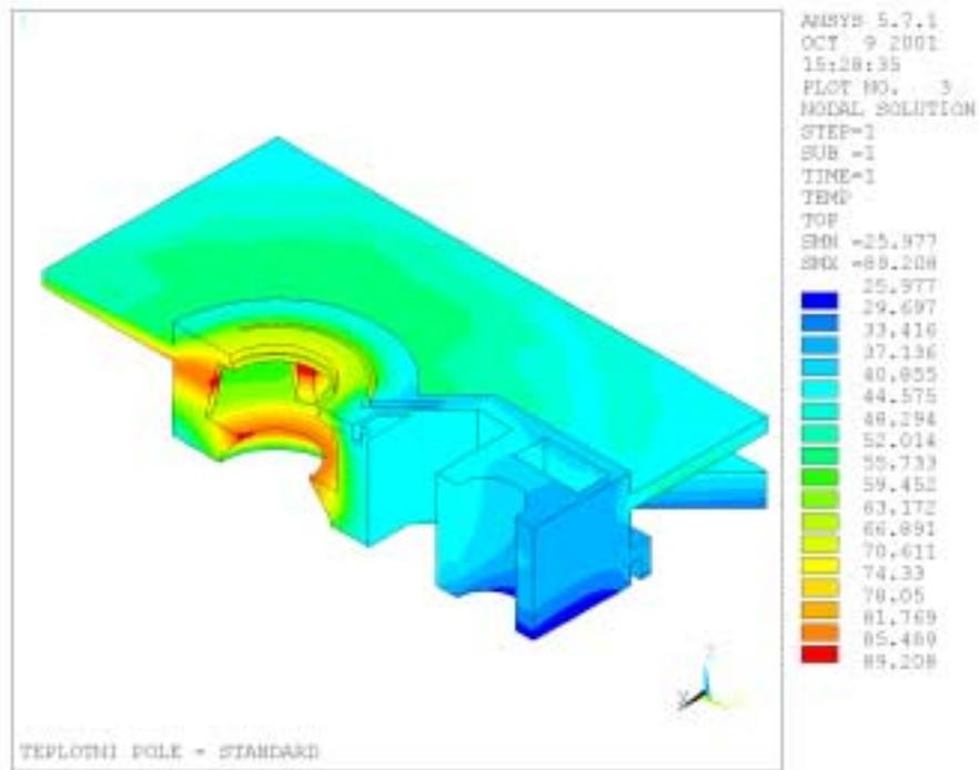
Fig. 2: Distribution of the temperature field on the concrete structures surface
