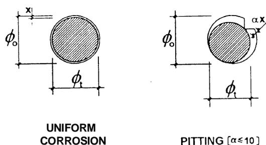
**Figure 5:** Residual steel section loss considered for the cases of uniform and localised corrosion.
