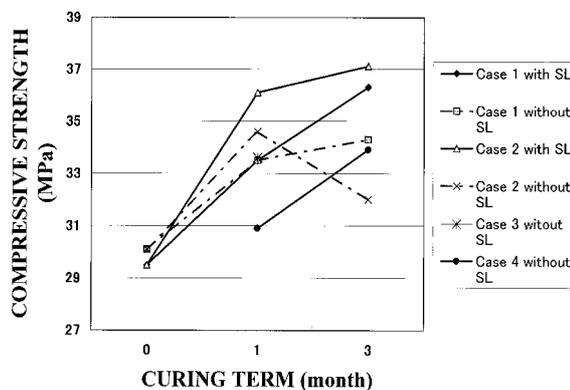
Fig. 16 Compressive strength of the mock-up concrete tests
