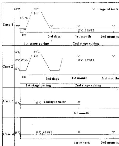
Fig. 15 Curing conditions of the mock-up test cases
