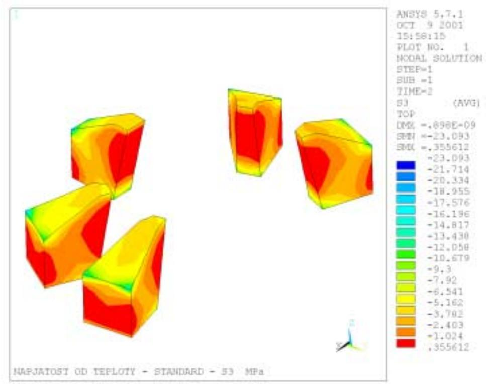
Fig. 3: State of stress (principal stress) of the concrete cantilevers initiated by the temperature loading
