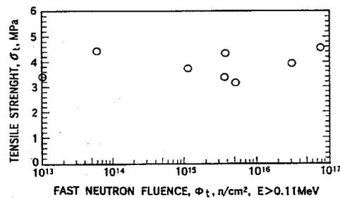
Fig. 14 Tensile strength along with fast neutron fluence
