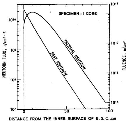
Fig. 3 Neutron flux and exposure dose distribution in the biological shielding concrete at the level of reactor core
