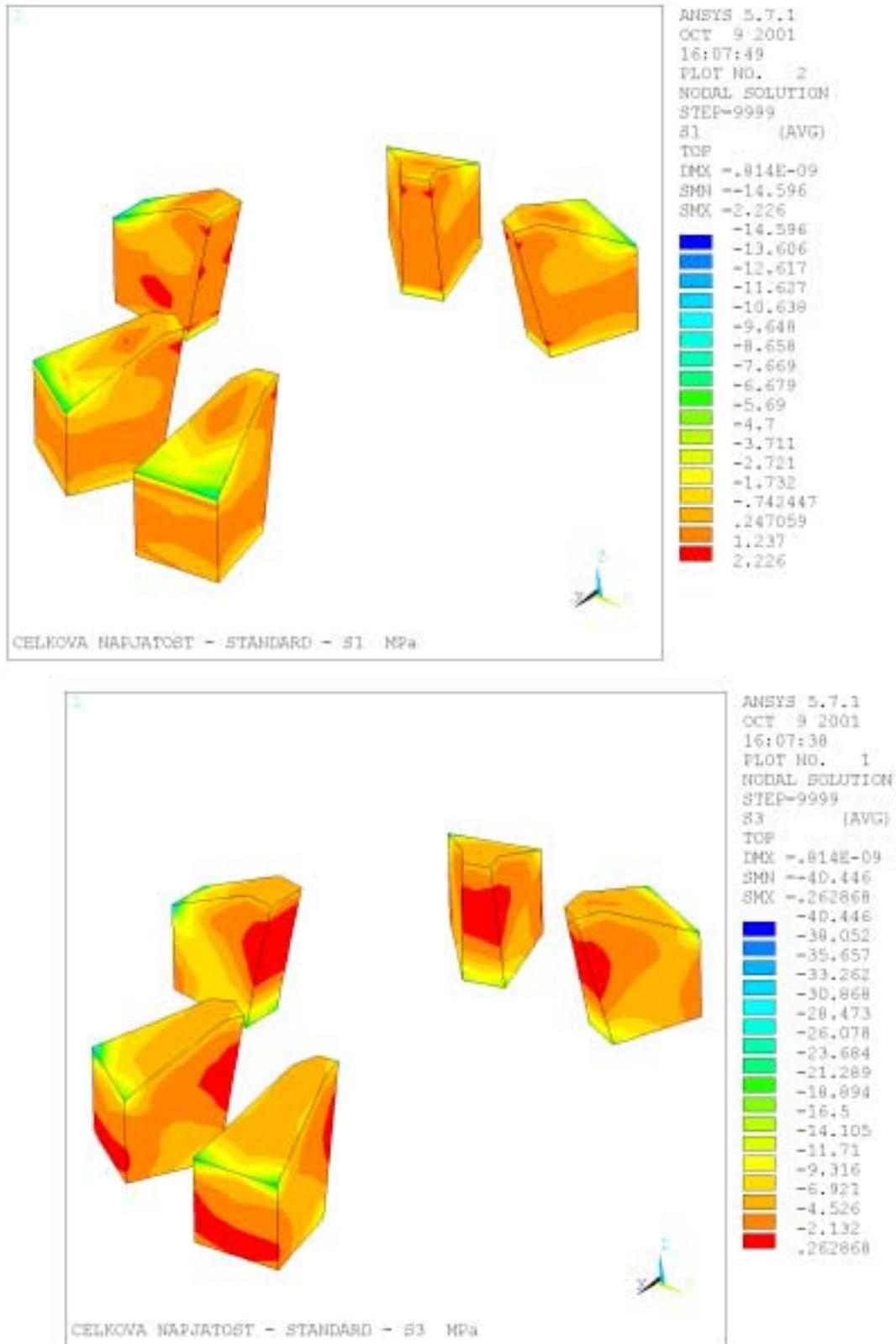
Fig. 4: Total state of stress (principal stress) of the concrete cantilevers (interaction of mechanical and temperature loading)
