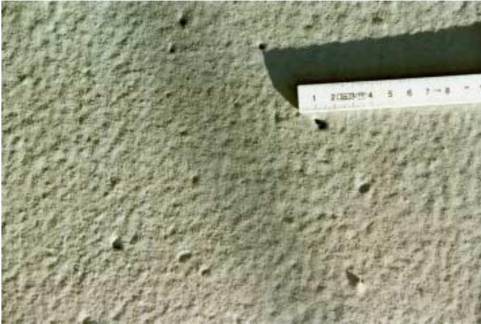
Picture 7: Surface of the crack – overbridging material with pores and hollows
