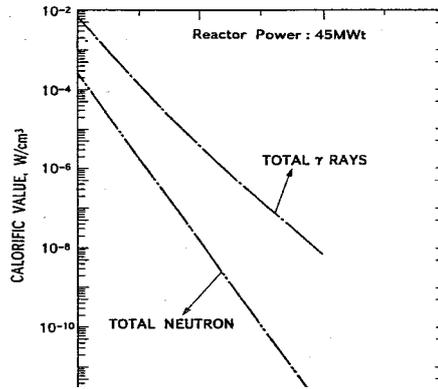
Fig.6 Calorific value distribution generated by total neutron and total gamma-rays at the level of reactor core
