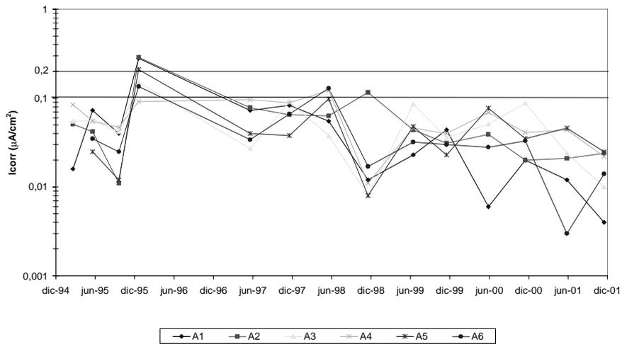
**Figure 4:** Results of  $E_{corr}$ , resistivity and  $I_{corr}$  measured during several years over an internal wall of the container.
