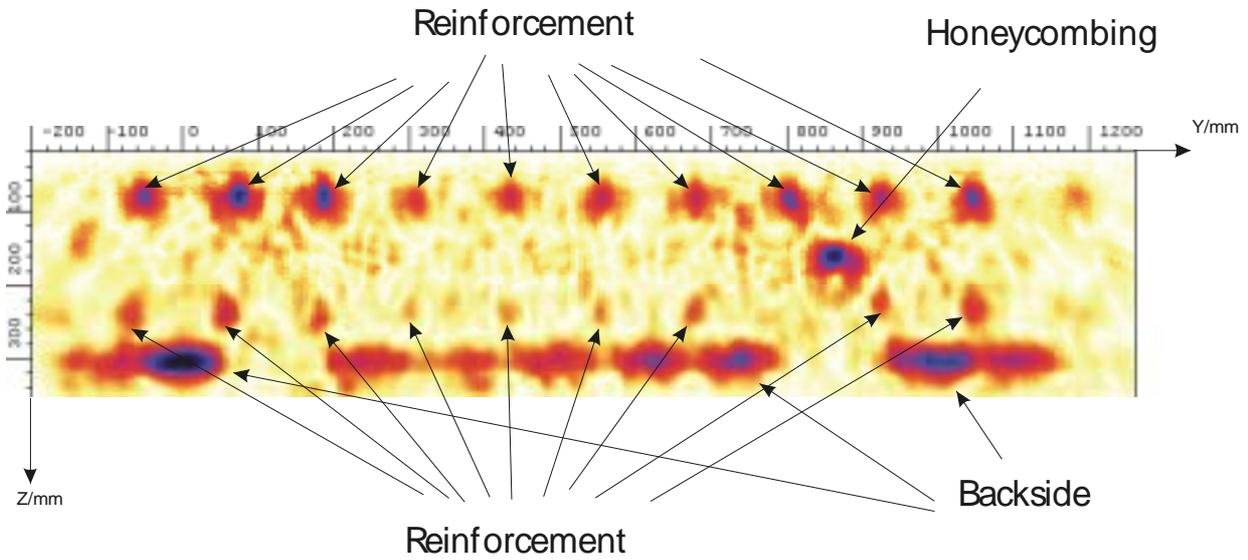
Fig. 7 3D-SAFT: B-Scan of base plate with reinforcement and two artificial flaws 88 mm x 34 mm
