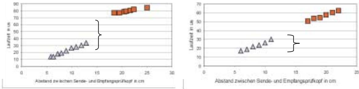
Air-filled crack; calculated depth: 91 mm      Water-filled crack; calculated depth: 22 mm
