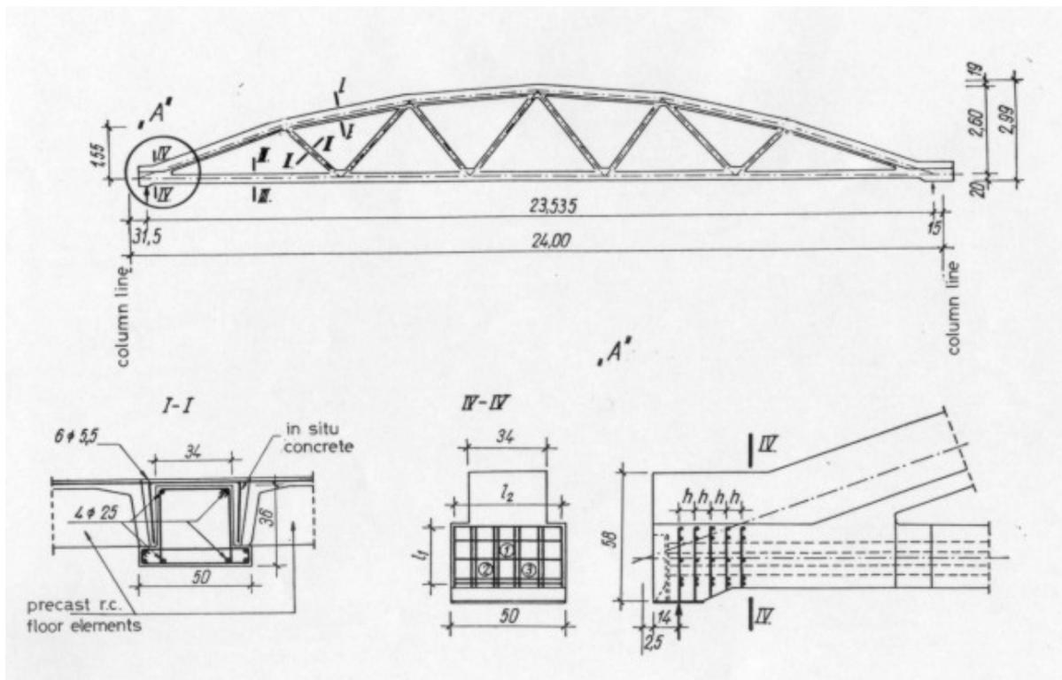
Fig. 1 The lay-out of the truss
