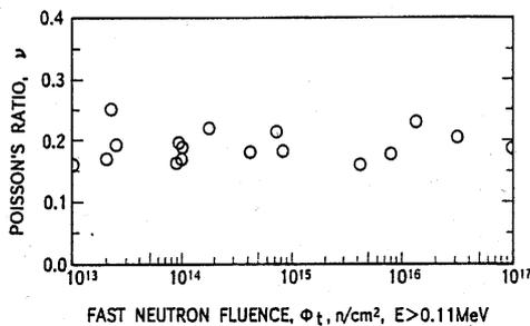
Fig. 13 Poisson's ratio along with neutron fluene
