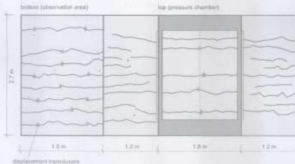
Fig. 8: Crack pattern of specimen 2
