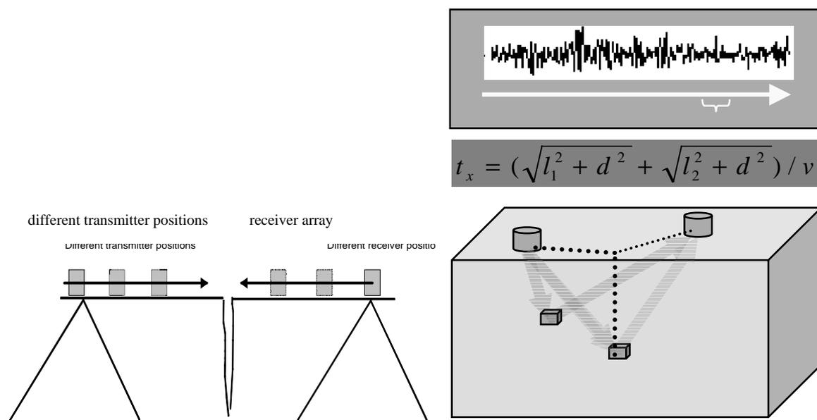
Fig. 3 Scanning arrangements for acoustic imaging with SAFT
