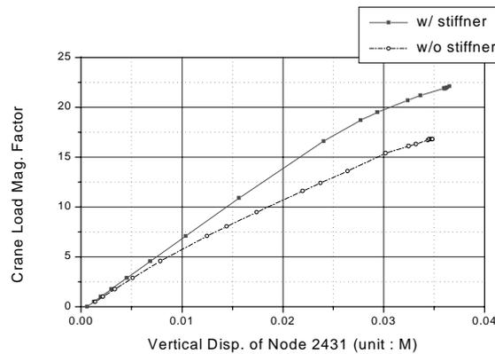
Fig. 4 The Relation of Crane Loading vs. Displacement at Node 2431
