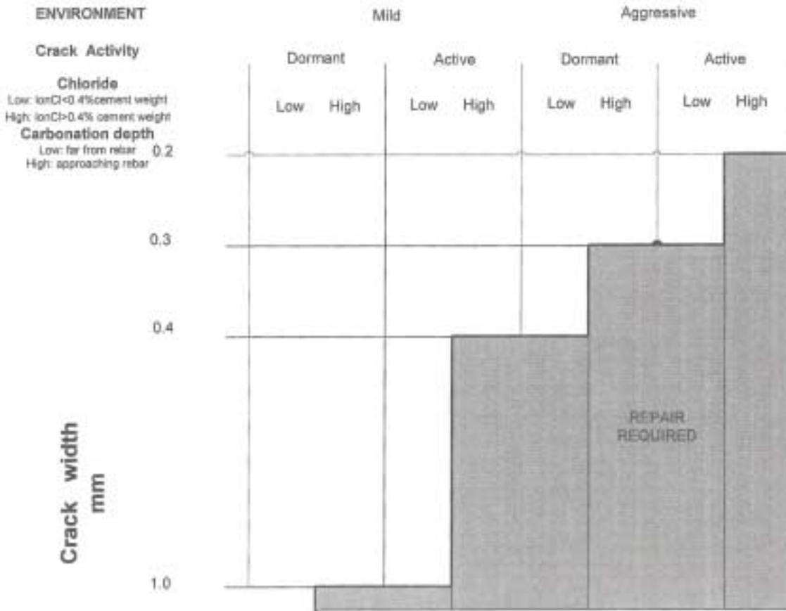
Fig. 2 Criteria for crack repair
