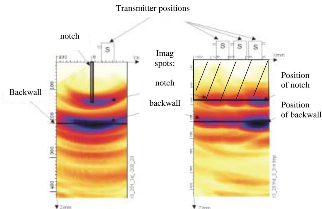
Fig. 4 Side View SAFT-images from a 150 mm deep empty notch
