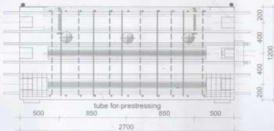
Fig. 7: Vertical section specimen type 2
