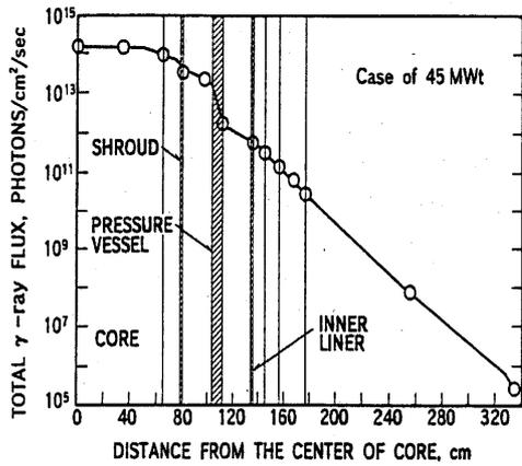
Fig.5 Distribution of total gamma-ray flux at the level of reactor core
