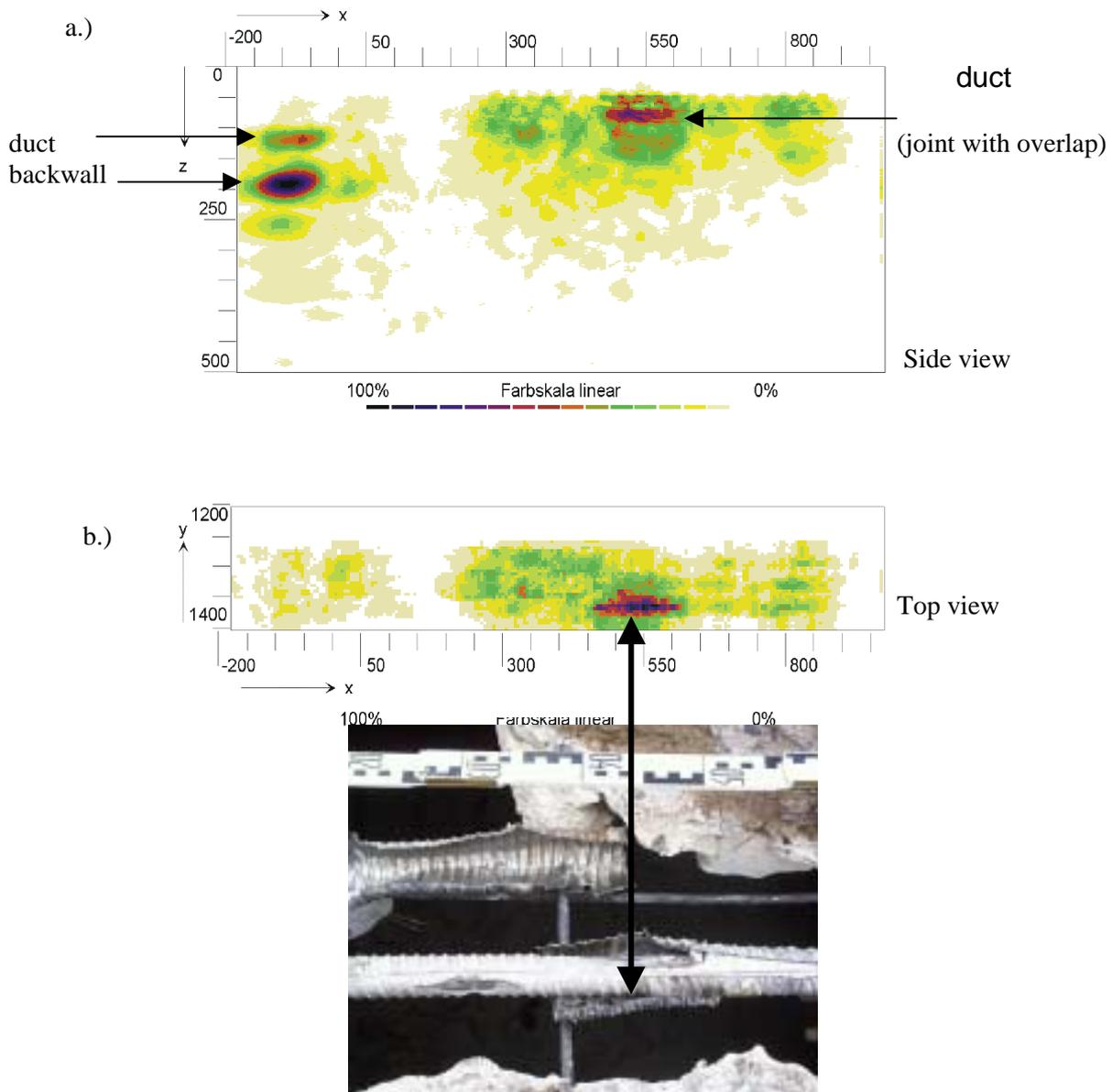
Fig. 8 Application of ultrasonic inspection on concrete motor way bridges
