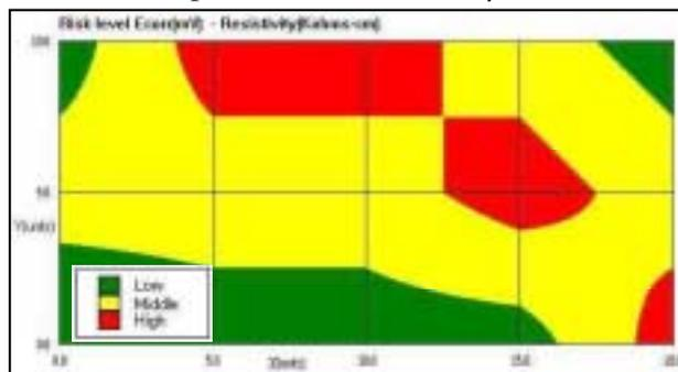
**Figure 1:** Corrosion risk map on a reinforcement slab calculated from the combination of Ecorr and  $\rho$  measurements.
