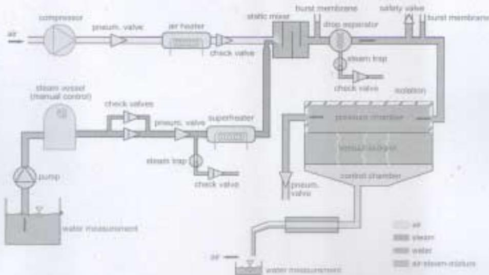
Fig. 5: Air-steam-mixture production principle
