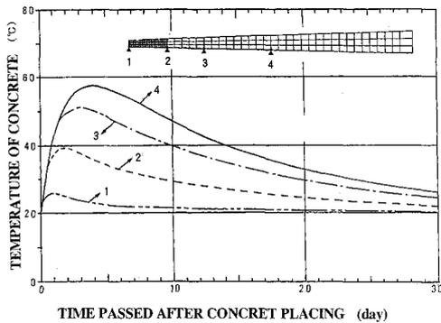
Fig. 7 Temperature distribution of the biological shielding concrete by the heat of hydration at the placing
