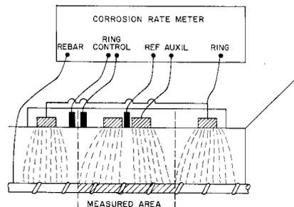
**Figure 2:** Modulated confinement of the current (guard ring) method
