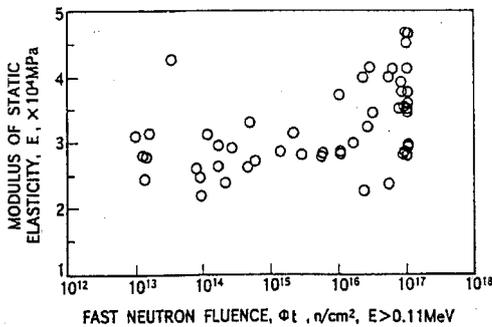
Fig. 11 Modulus of static elasticity along with fast neutron fluence
