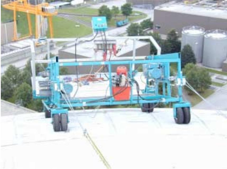
Picture 6: **New designed light weight scaffolding/platform**
