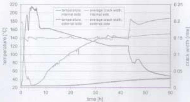
Fig. 9: Temperature and crack width specimen 2/2
