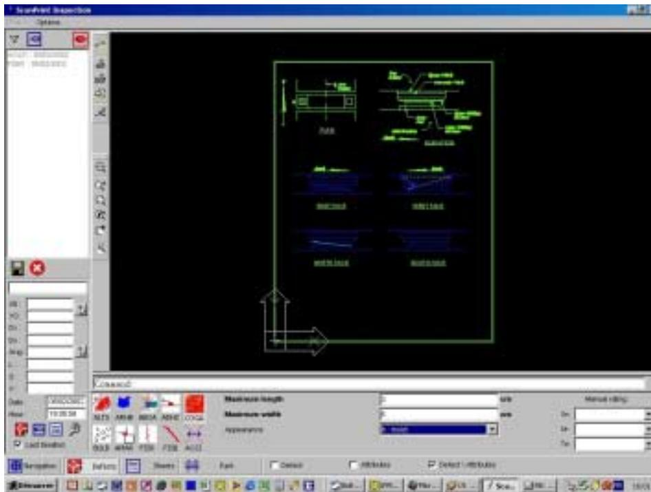
**Fig.4: Site inspection software running on pen-touch computers**
