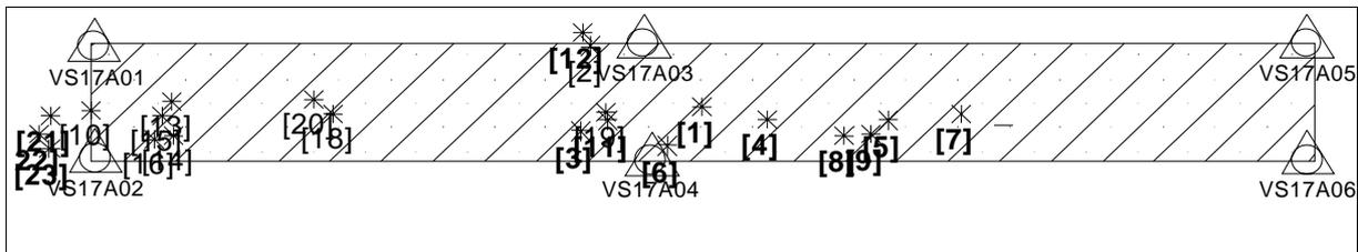
Figure 7 – Location of Events from 30 kN to 100 kN (6,700 lbf to 22,500 lbf)
