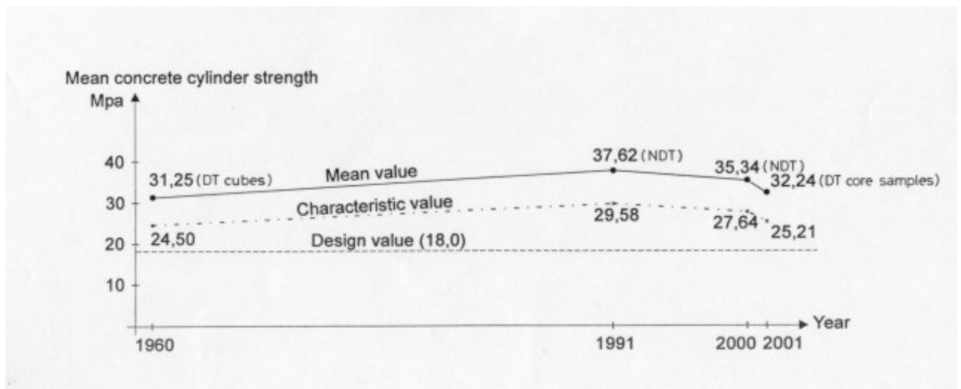
Fig. 3 Concrete strength variation in time
