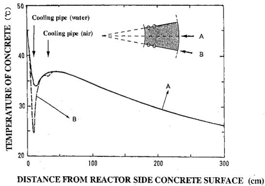
Fig. 8 Temperature distribution of the biological shielding concrete in the operation
