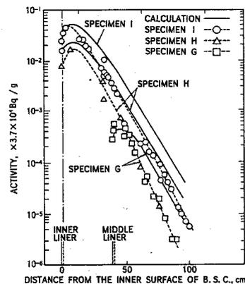
Fig. 4 Activity distribution in the biological shielding concrete at the level of reactor core (Eu-152)
