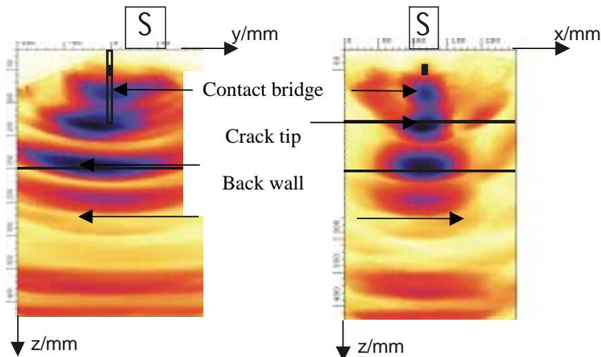
Fig. 5 Correct depth sizing despite a contact spot in the notch due to SAFT-application
