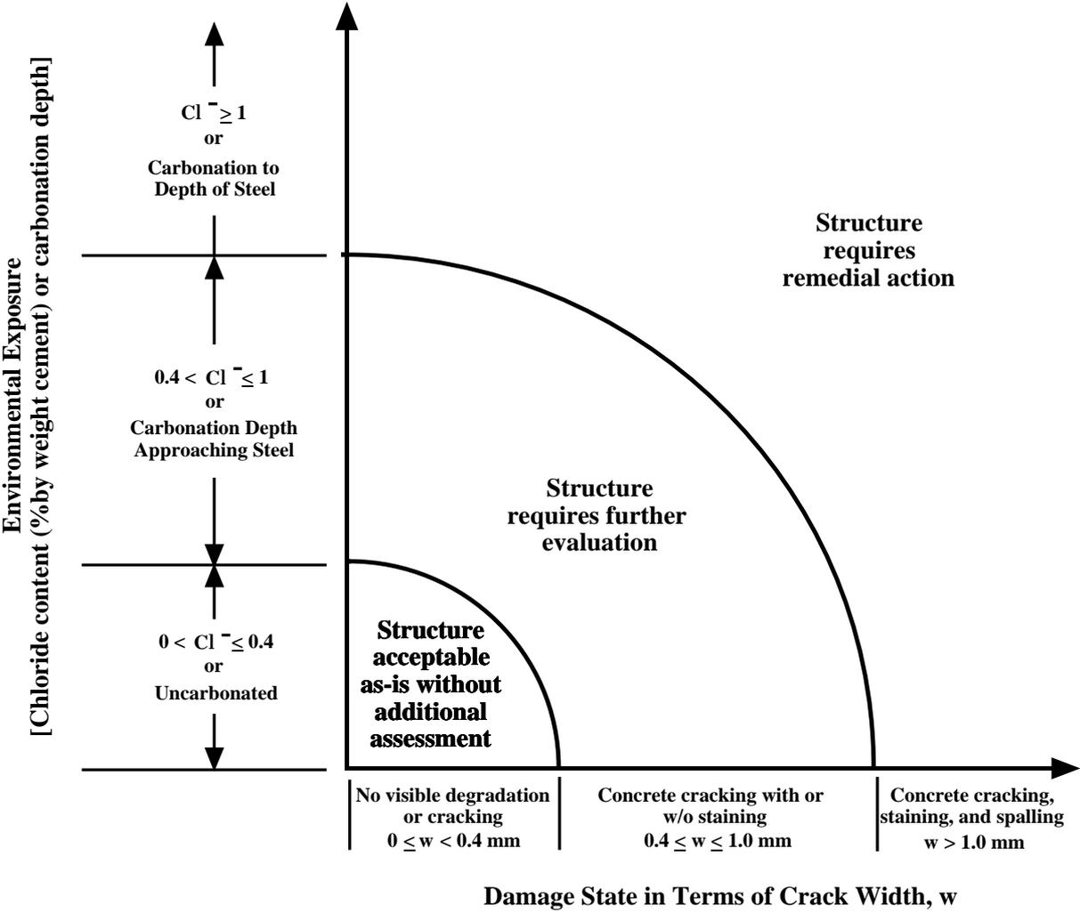
FIG. 7.3. Damage state chart relating environmental exposure, crack width, and necessity for additional evaluation or repair [Ref. 7.6].
