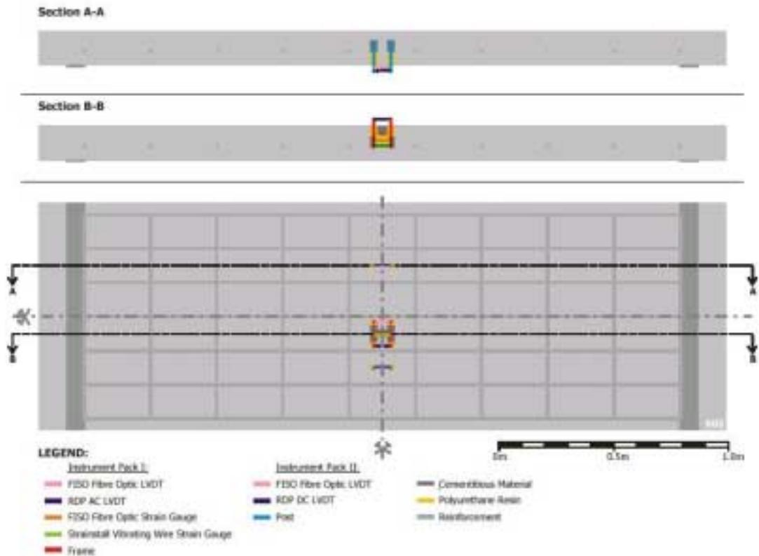
Figure 2 Layout of the instrumentation employed on beam for stage 2 (extension)
