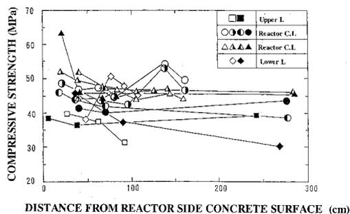
Fig. 9 Compressive strength along with concrete depth
