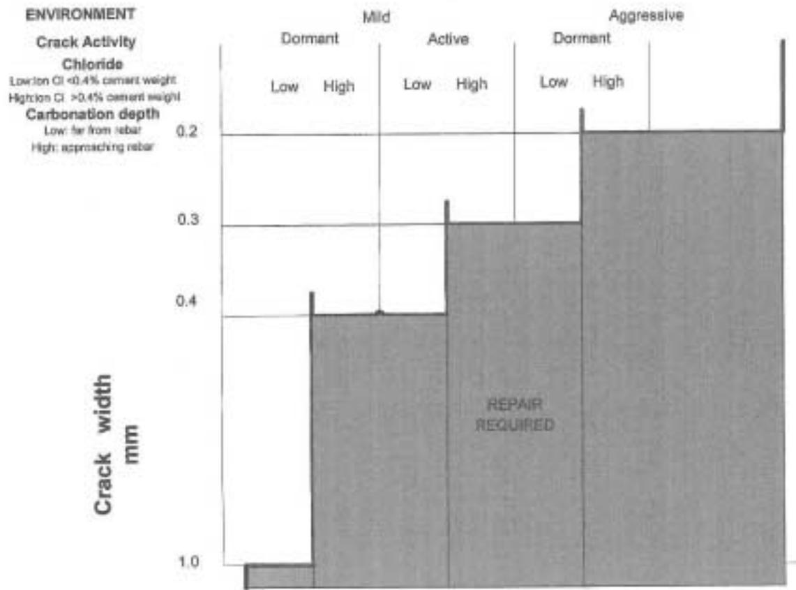
Fig. 1 Criteria for crack repair
