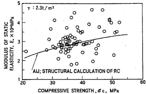
Fig. 12 Relationship of compressive strength and modulus of static elasticity
