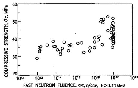
Fig. 10 Compressive strength distribution along with fast neutron fluence
