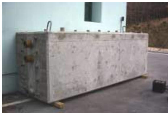
Photograph 1. Prototype Structural Member of Containment Building Of Nuclear Power Plant
