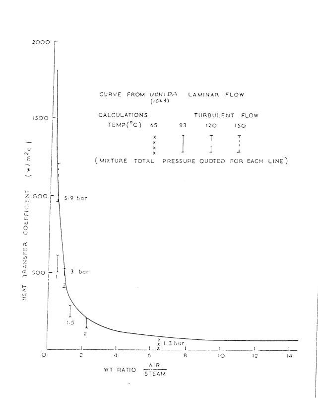
FIG. 1 HEAT TRANSFER WITH CONDENSATION FROM STEAM-AIR
