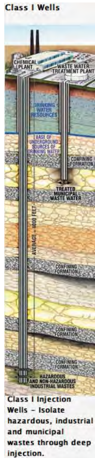
Figure 5.4-3: Deep well injection techniques for hazardous and toxic waste fluids ( http://water.epa.gov/type/groundwater/uic/wells_class1.cfm#what_is )
