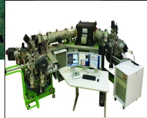
Large geometry secondary ion mass spectrometry (SIMS)
