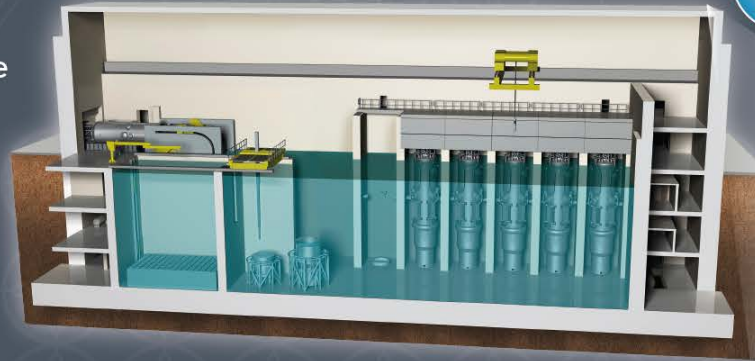
Housed in a 12 module reactor building
