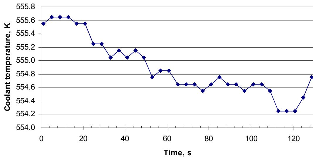
**Table C.7. Cold leg #2 coolant temperature during the transient**
