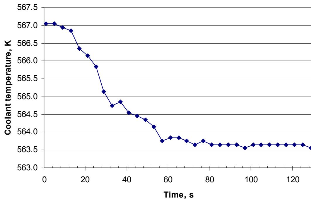
**Table C.11. Hot leg #2 coolant temperature during the transient**
