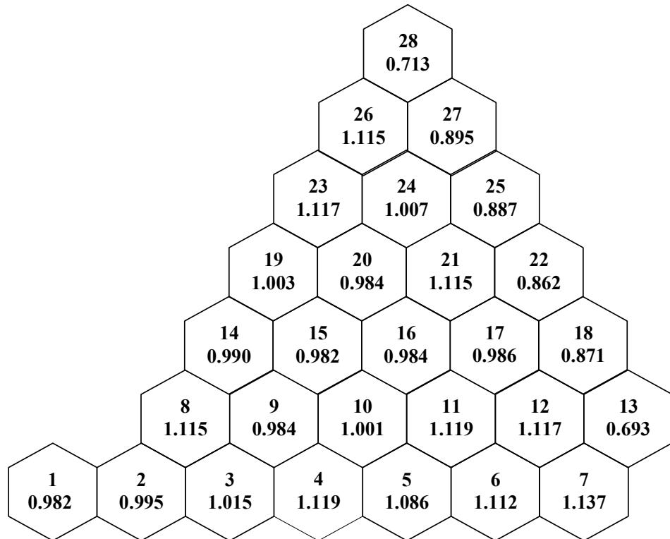
**Figure 5.3.2. Initial HP core average axial relative power distribution**
