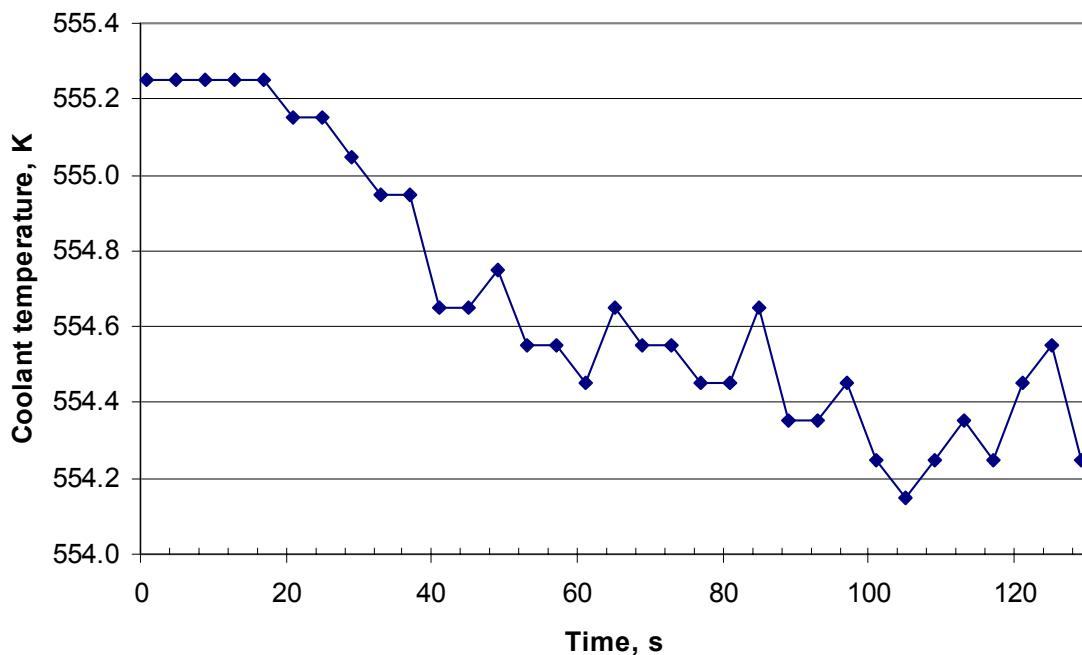
**Table C.10. Hot leg #1 coolant temperature during the transient**
