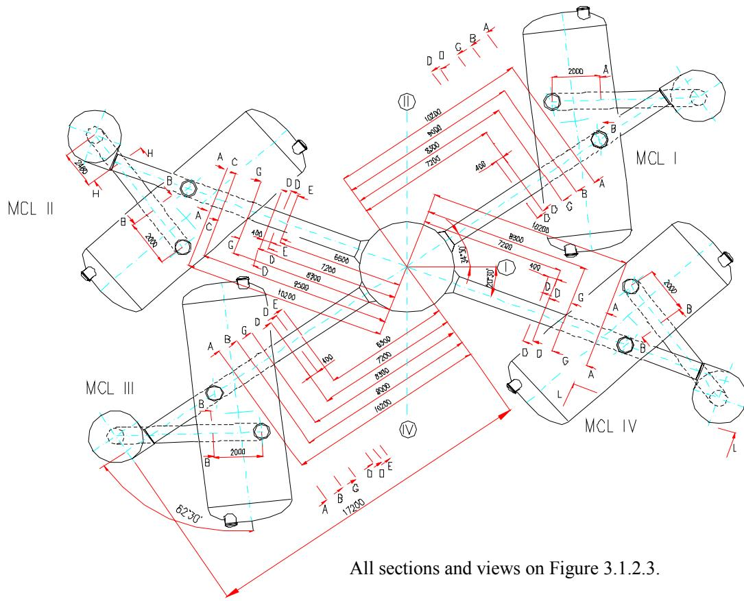
**Figure 3.1.2.3. Primary circuit layout 2**
