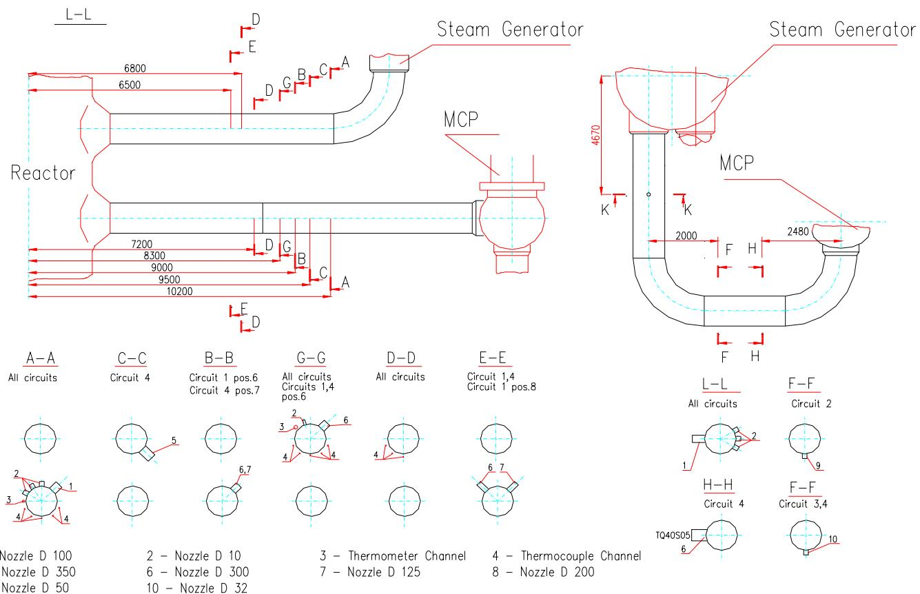
**Figure 3.1.2.4. Main equipment layout**
