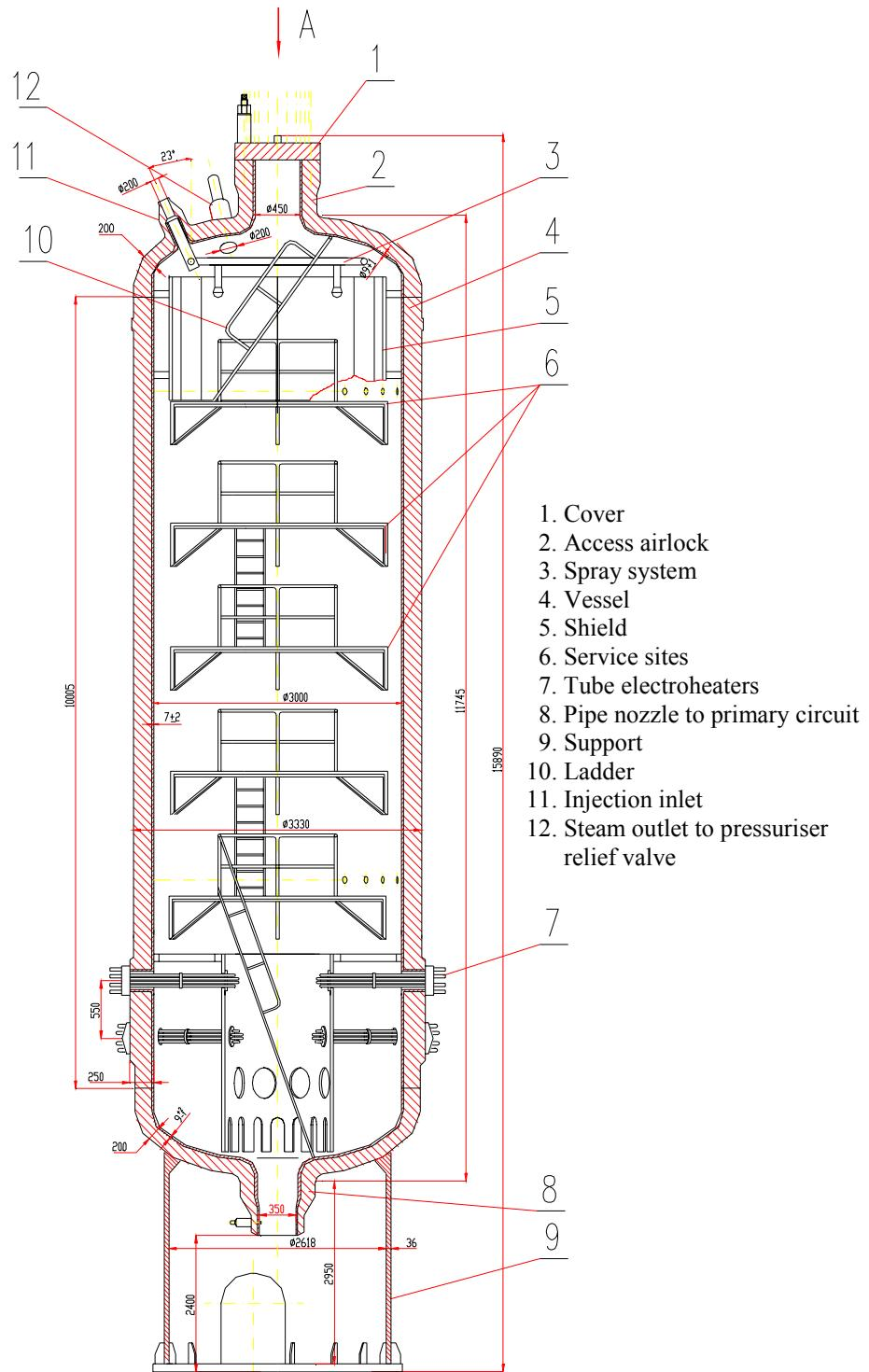
**Figure 3.1.2.7. Pressuriser cross-section**
