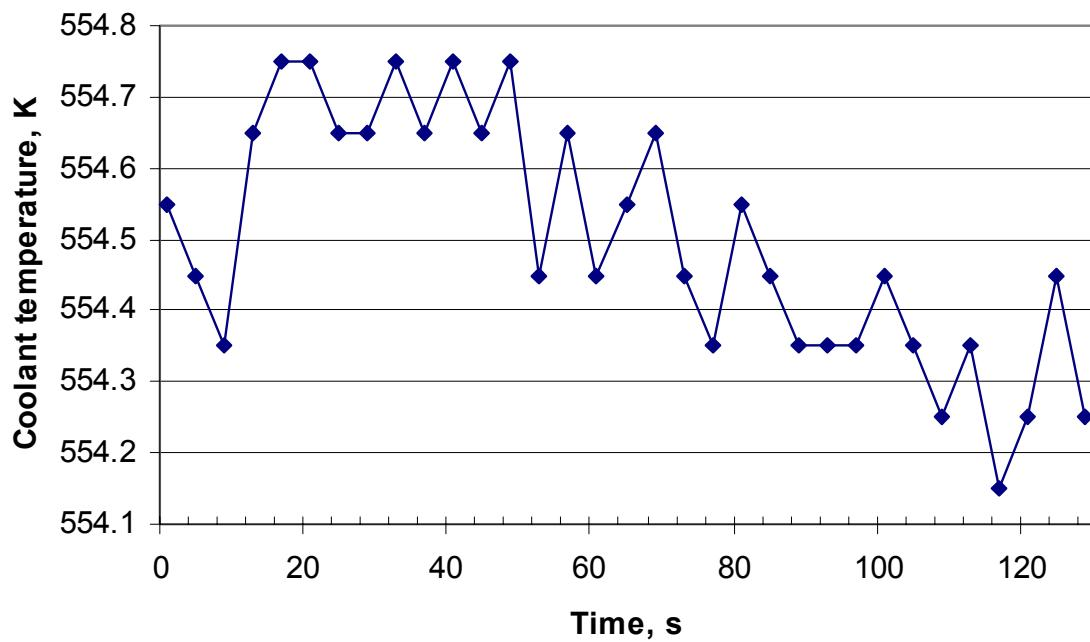
**Table C.8. Cold leg #3 coolant temperature during the transient**
