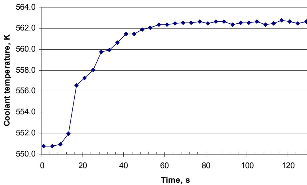
**Table C.13. Hot leg #4 coolant temperature during the transient**
