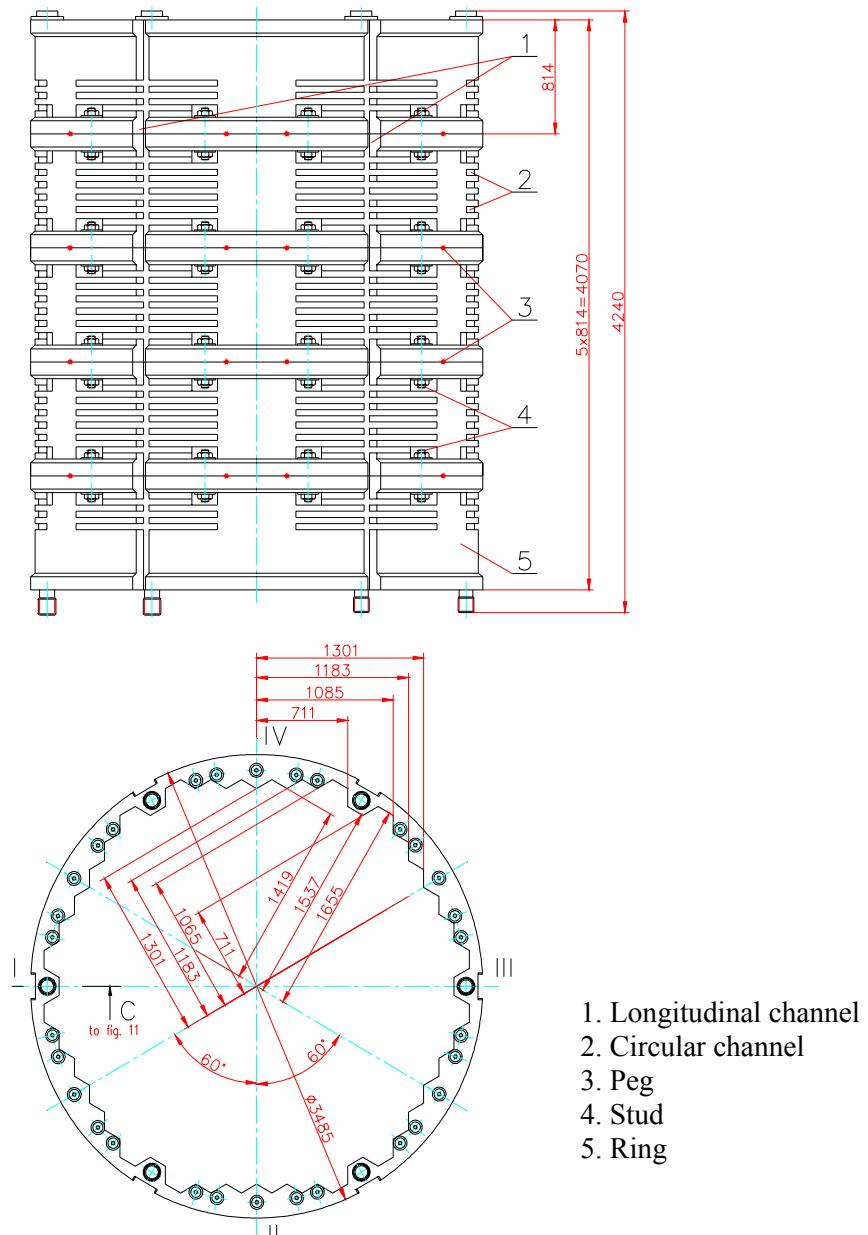
**Figure 3.1.1.6. Reactor shielding tubes block**
