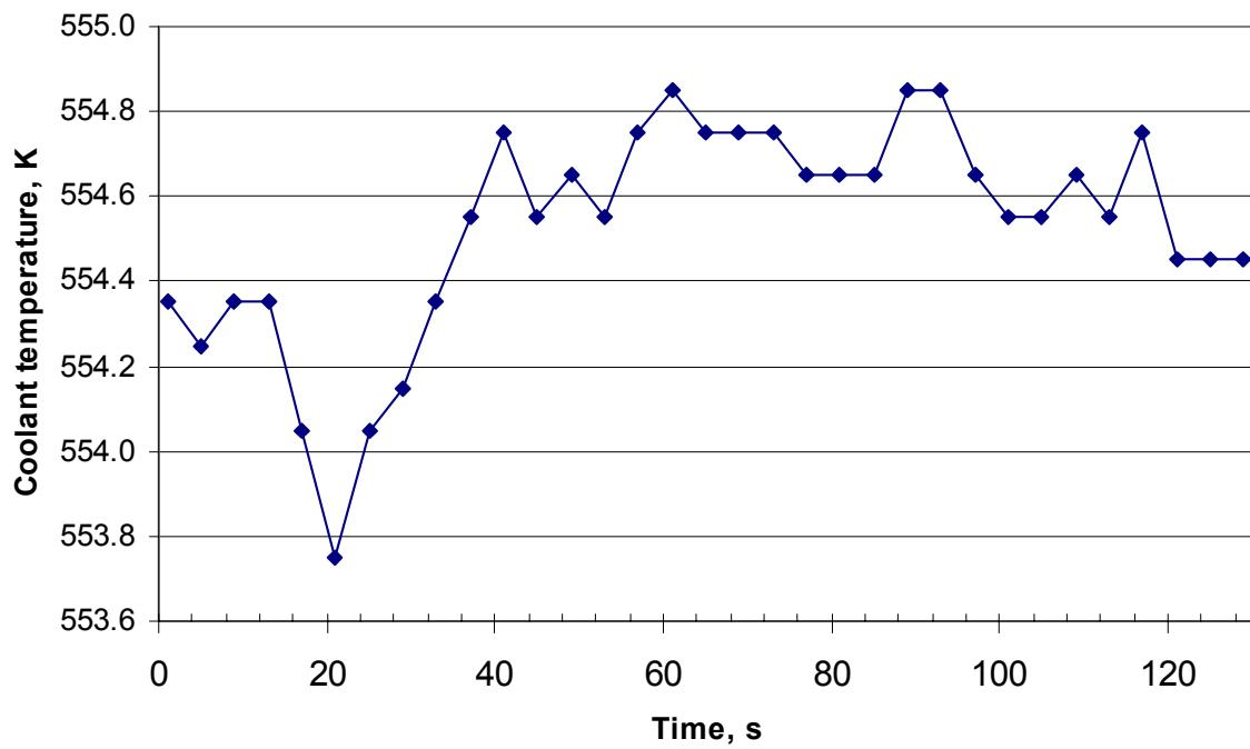
**Table C.9. Cold leg #4 coolant temperature during the transient**
