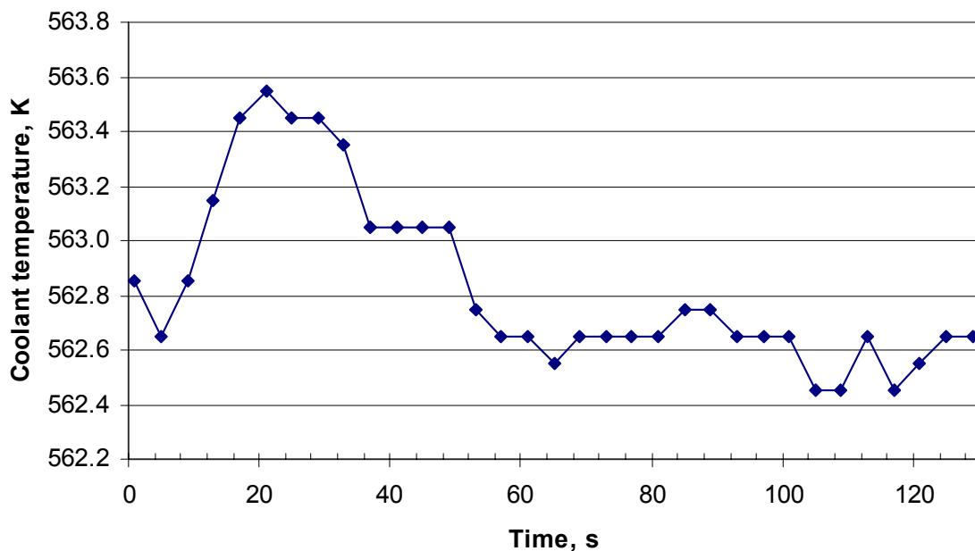
**Table C.12. Hot leg #3 coolant temperature during the transient**
