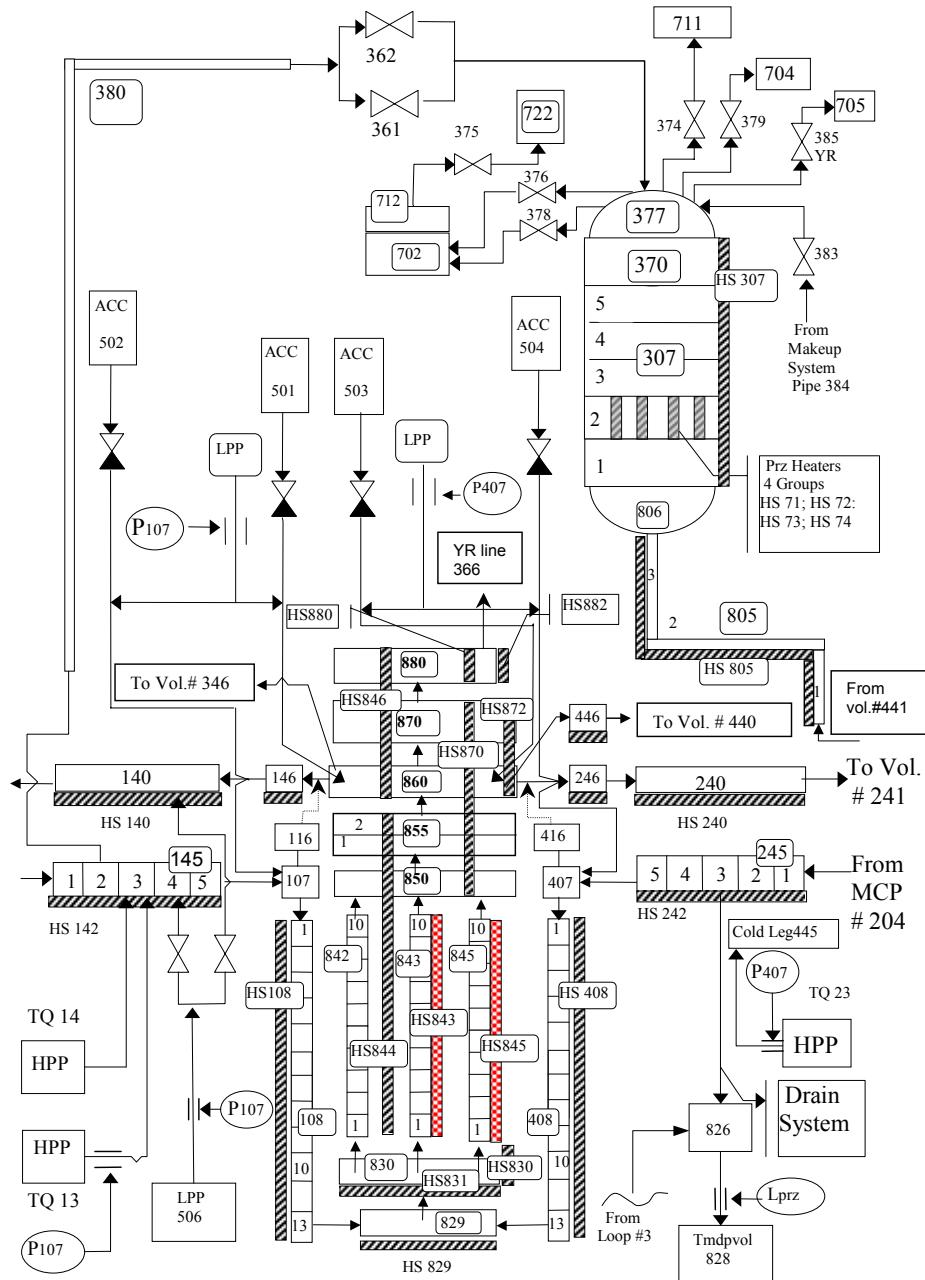
**Figure A.2. VVER-1000 Unit 6 steam generator RELAP5 four loops model**
