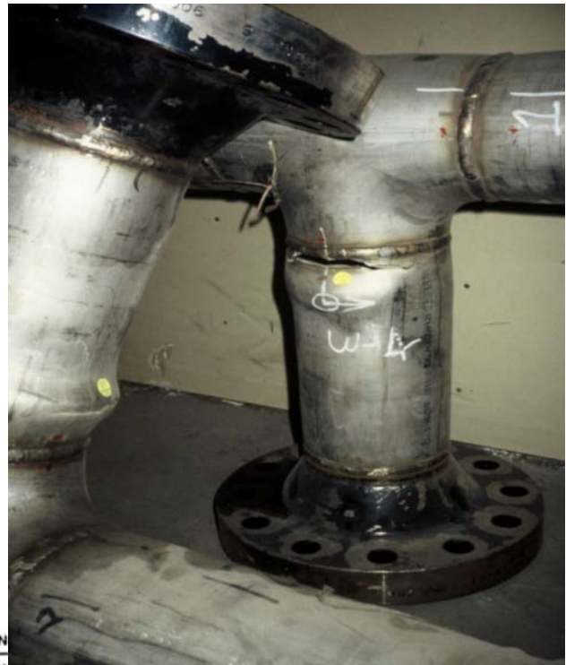
Figure 2: Ratchetting effect (swelling) observed on a component
