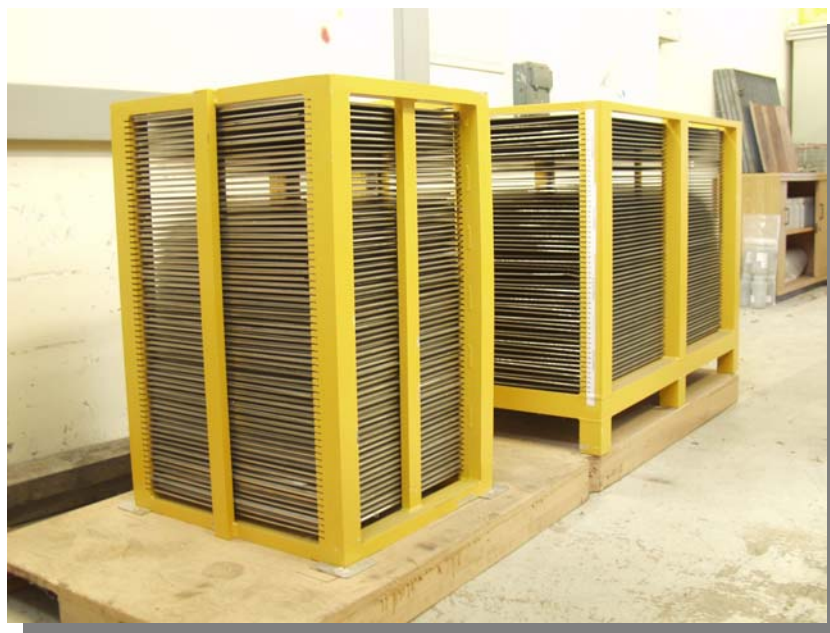
Figure 2: Calibration racks for release measurements facilities
