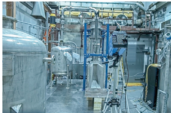
Test facility for ROSAU corium melts spreading tests. Argonne National Laboratory (ANL), United States
