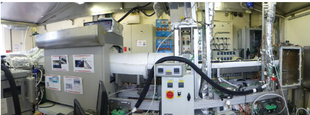
CHIP experimental facility to study fission product transport and deposition in the primary circuit. IRSN, France
